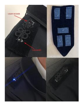
Figure 33. Light sensor with LED-light on right shoulder pad.
