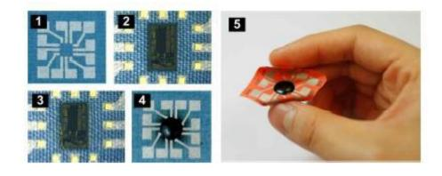
Figure 10. Single-layered P-FCB system manufacturing process [12].
