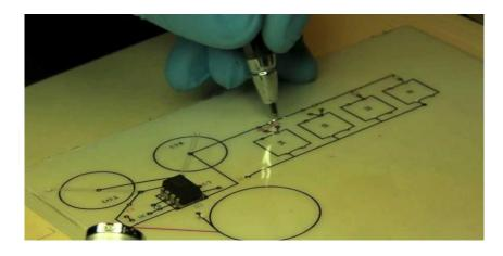
Figure 8. Drawing with conductive ink [12].
