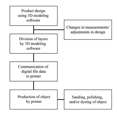
Figure 12. General design and production process of 3DP methods [18].
