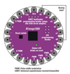
Figure 13. Diagram of the Lilypad microcontroller module [21].
