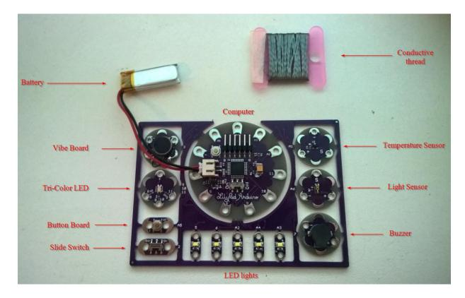
Figure 20. Lilypad Arduino when received
