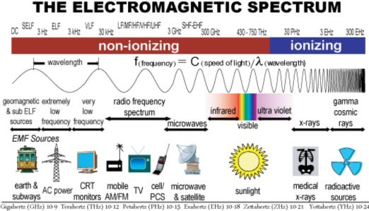
Figure 14. Electromagnetic spectrum [30].
