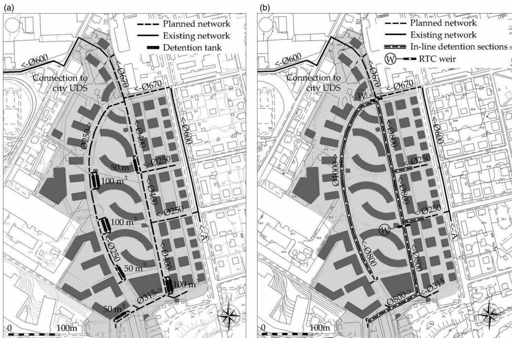
Figure 6 | Technical solutions for the peak flow reduction: (a) off-line detention tanks; (b) in-line detention with RTC.
