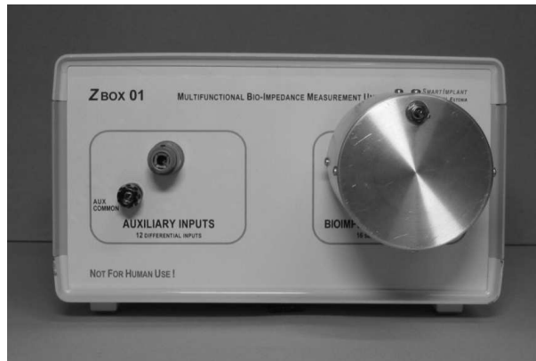
Fig. 56. Instrument with test fixture (aluminum enclosure on the right) attached.
