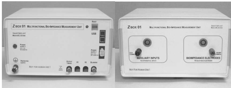
Fig. 54. Outside view of the first device, front view in the left, and backside on the right.
