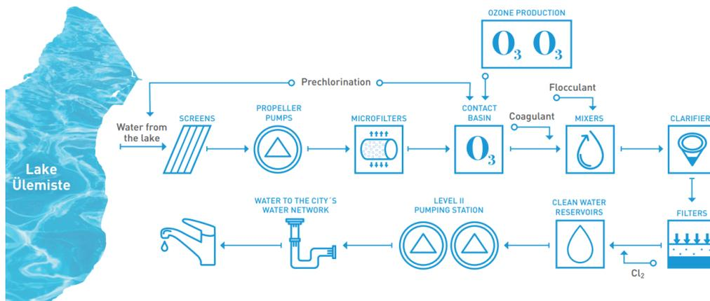
Figure 8. Water treatment process at Ülemiste Water treatment plant (Tallinna Vesi AS, 2022)
