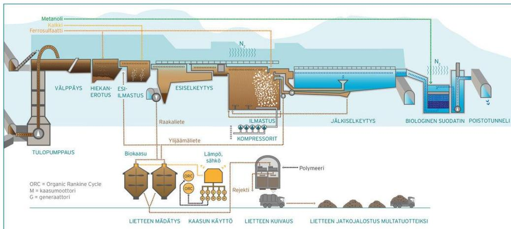
Figure 27 Wastewater treatment process at the Viikinmäki station (HSY, 2022)
