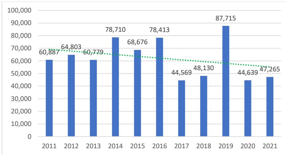
Figure 30. Combined CO<sub>2</sub> emissions from WWTPs in Helsinki, tons (HSY Statistics Department, 2023)
