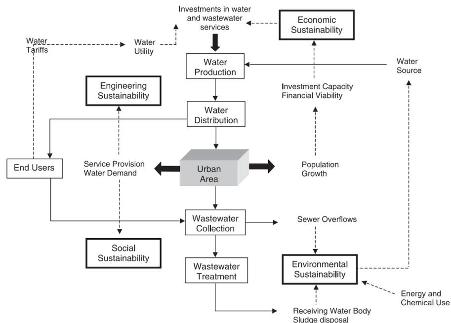
Figure 6. Urban water sector system. Solid lines represent water flows, and broken lines represent relevance to sustainability (adapted from Sahely et. al 2005).
