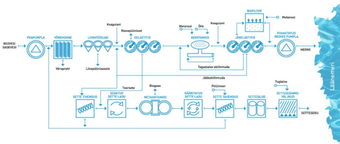
Figure 10. Wastewater treatment process at Paljassaare wastewater treatment plant (Tallinna Vesi AS, 2021)
