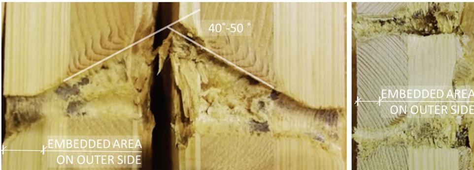
Figure 63. Left: embedded area of long SBD; right: the same for long WS
