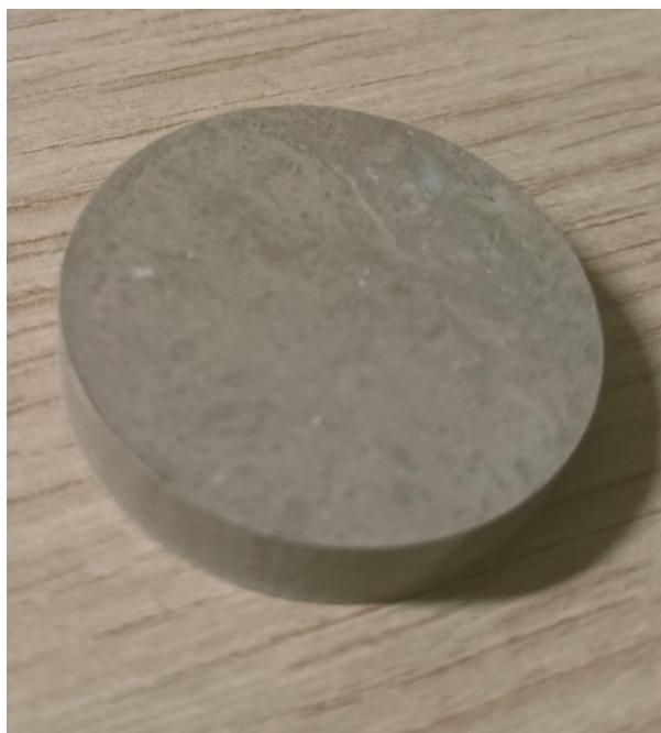
Figure 8. Example of a pressed sample pellet with a diameter of 32 millimetres.
