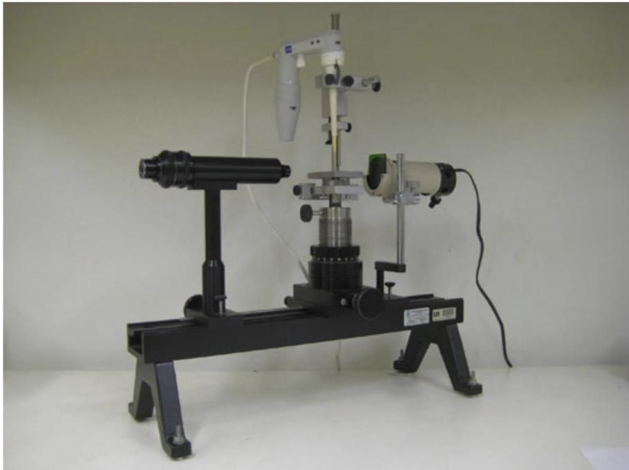
Figure 2.4 A ramé-hart contact angle goniometer:
