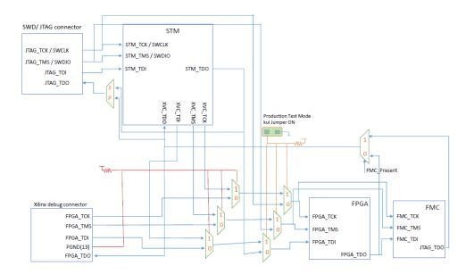
Figure 26. JTAG/SWD block schematic
