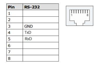
Figure 7. RS-232 RJ45 connector layout
