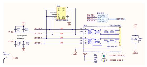
Figure 11. RJ45 schematics
