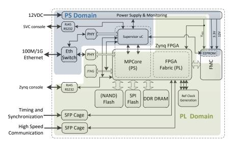
Figure 16. FPGA IOC power domains
