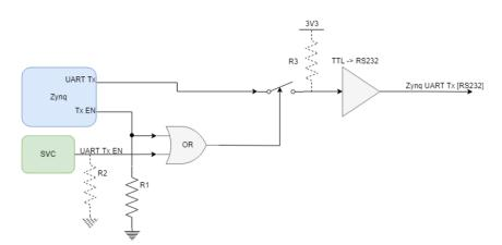
Figure 6. Enabling or disabling the Zynq TX line with analog switch
