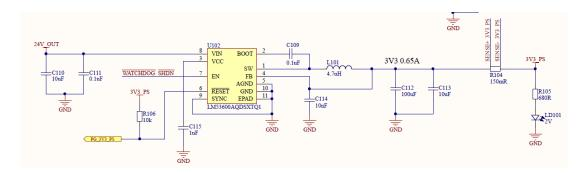
Figure 21. 3.3V\_PS DC/DC converter
