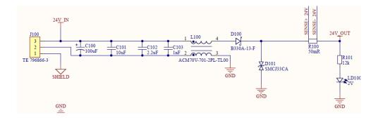
Figure 18. Input protection of the FPGA IOC power domains
