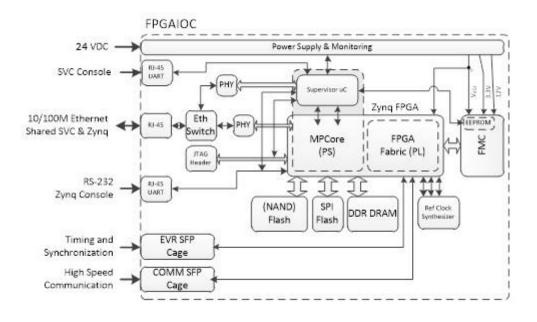
Figure 2. System Architecture sketch of FPGAIOC
