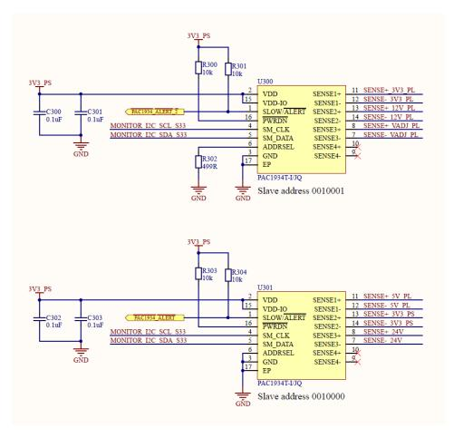
Figure 25. PAC1934 power monitoring schematics
