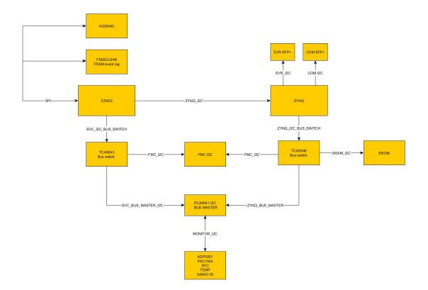
Figure 15. I2C and SPI block diagram
