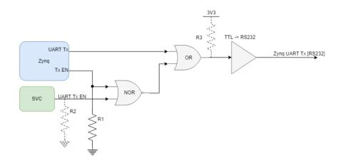
Figure 5. Enabling or disabling the Zynq TX line with logic gates
