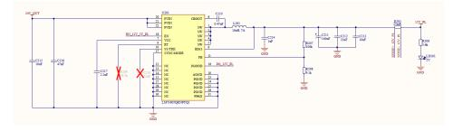
Figure 23. 12V\_PL rail DC/DC converter
