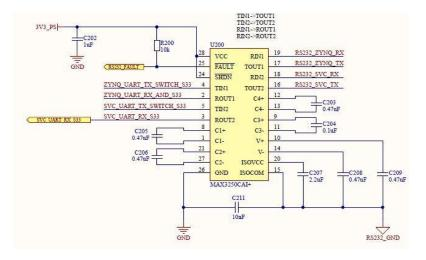
Figure 8. MAX3250 schematic
