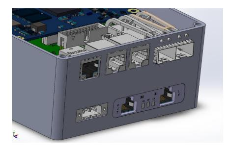
Figure 27. FPGAIOC connectors and PCB placement
