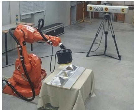
Fig. 2. Scanning by Nikon K-Robot scanning system
