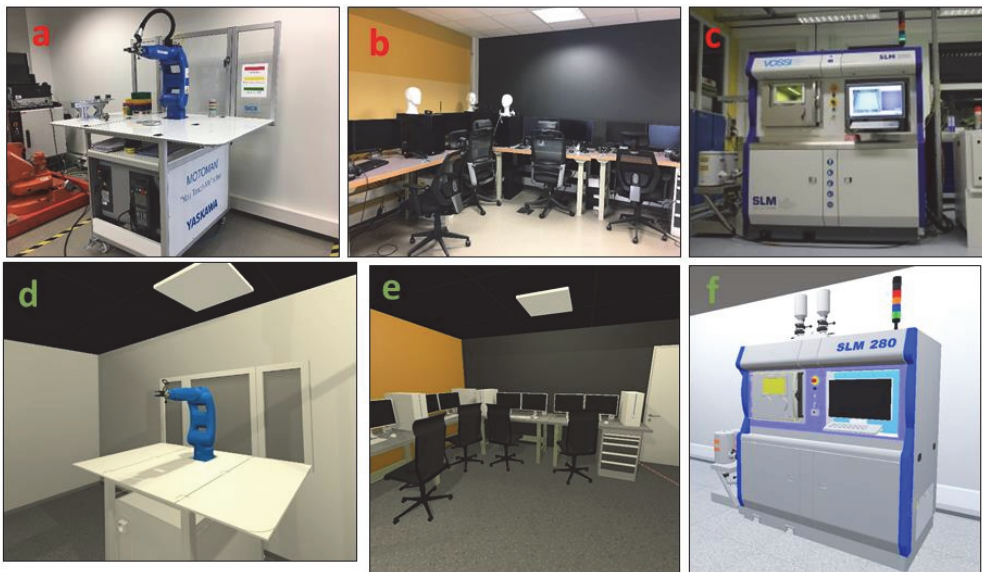
Figure 1. Digitalized laboratory – FMS and Robotics Demo Centre and ProtoLab (a, b, c – real; d, e, f – replica)
