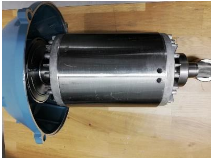
Figure 4.4. Two broken rotor bars
