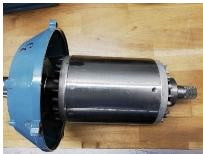
Figure 4.3. One broken rotor bar
