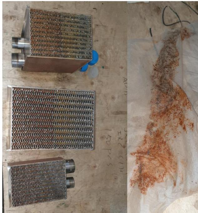
Figure 3.14. DHW-HEX in three pieces (left) and contents (right)
