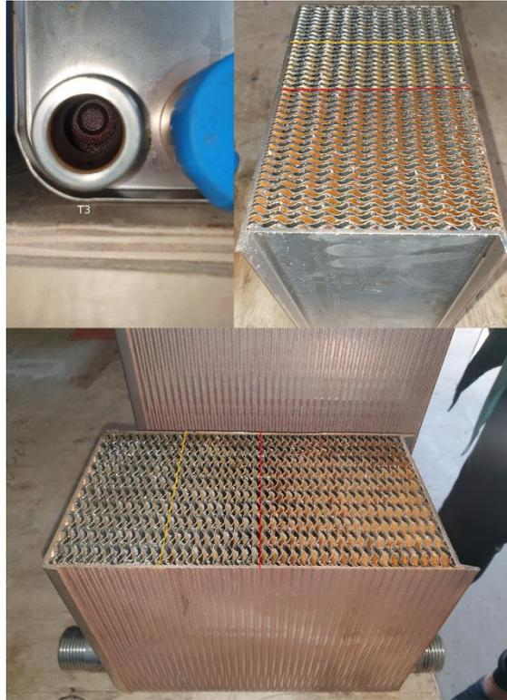
Figure 3.15. Contamination of 2S-HEX by DHW in Tallinn after operating for 1 year and 4 months
