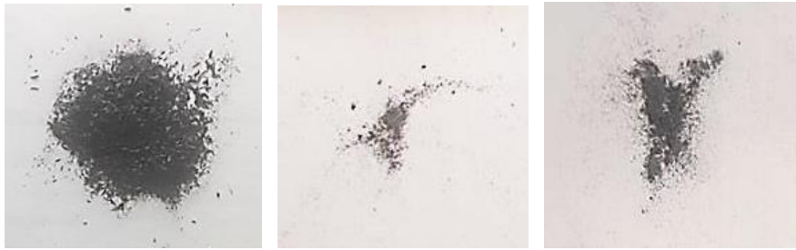
Figure 26. Solid residues from spruce at 750 °C (left), 850 °C (center) and 950 °C (right)
