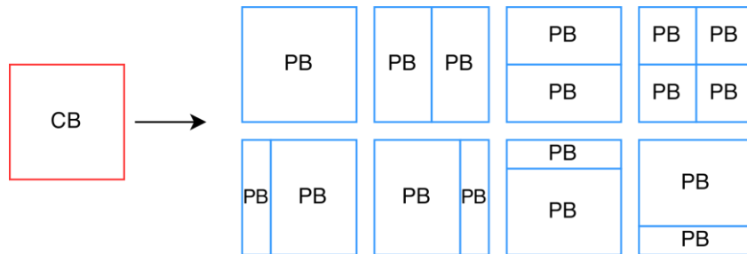
Figure 4. Different ways to divide a CB into PBs
