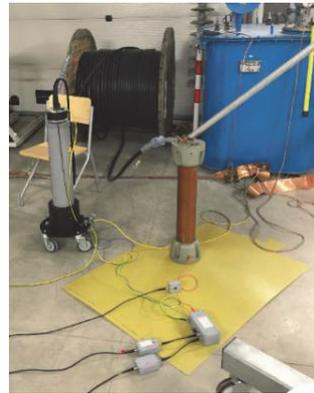
**FIGURE 10.** Laboratory test setup for online measurement of PDs in the MV cable (physical layout).
