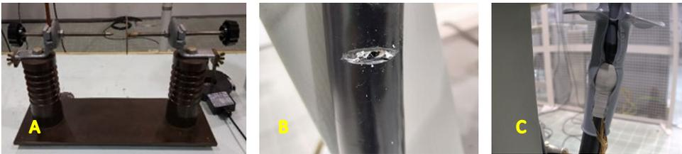
Figure 30. Partial discharge sources used in the tests to distinguish different types of PD: A) corona discharge, B) internal discharge, C) surface discharge
