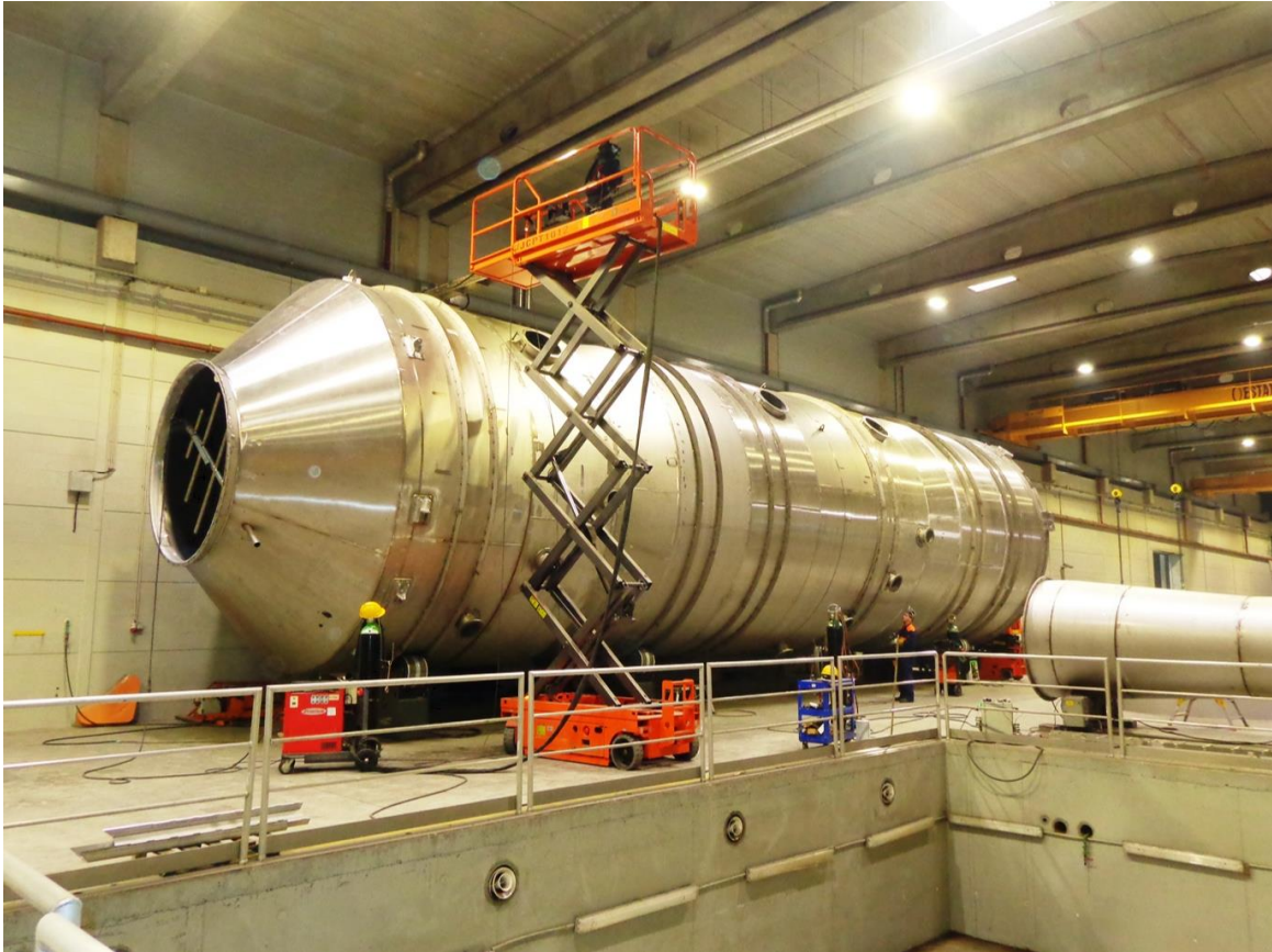
Joonis 2.3 Marine Scrubber. Outer shell diameter: 5,6 m Height: 20 m Dry weight: 38,5 t Number of details: ca 5000. Main shell materials: EN no 1.4529 (alloy 926); 1.4547 (254SMO), 2.4605 (alloy 59) ja 1.4410 (Super Duplex) [1]
