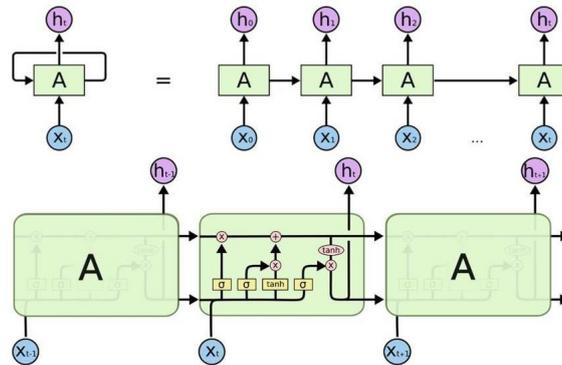
Figure 4. *RNN neural network architecture with LSTM cell. Source: [14]*
