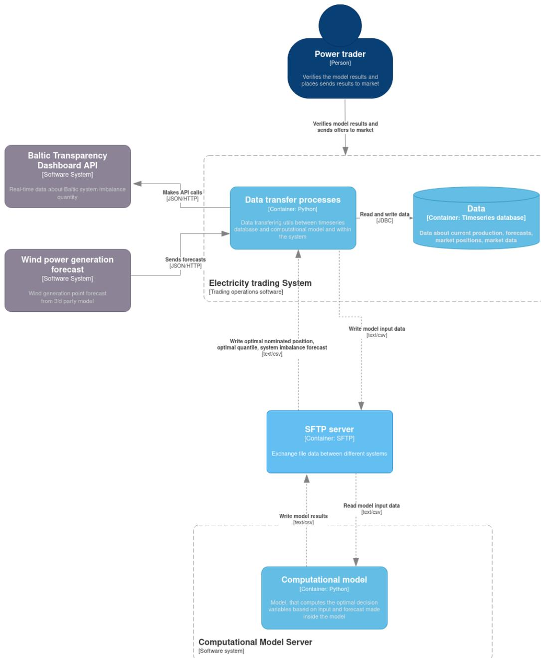
Figure 12. Component architecture diagram illustrating inputs and outputs of the model
