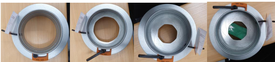
Figure 2.4 Regulator damper setpoints K=0 , K=4 , K=8 , K=8 with tape
