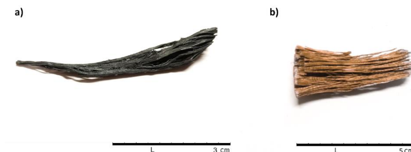
Figure 18: Photograph of a) final synthesis product of dip coating approach b) Final Product of Wet Combustion Synthesis Using Glycine as Fuel
