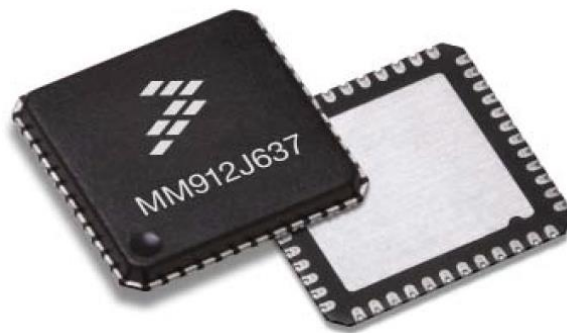
Joonis 2.8. Freescale MM912 637© 98ASA00343D korpuses[7]
