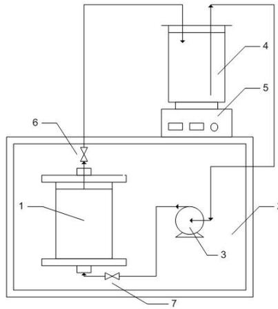
**Figure 5.** Laboratory set-up for coupled aerobic/anaerobic SBR (CSBR). 1-anaerobic reactor, 2-thermostat, 3-peristaltic pump, 4-aerobic reactor, 5-magnetic stirrer, 6 and 7 - valves
