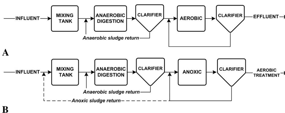
**Figure 3.** Initial and modified treatment schemes. **A** - original scheme for baker's yeast wastewater treatment (OY Tampella AB, Finland), **B** - modified anaerobic/anoxic scheme proposed and adapted by author at the beginning of experiments
