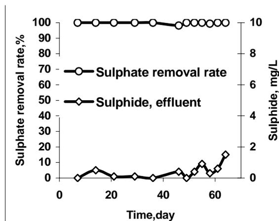
**Fig. 2.** Sulphate removal efficiency during the experiment
