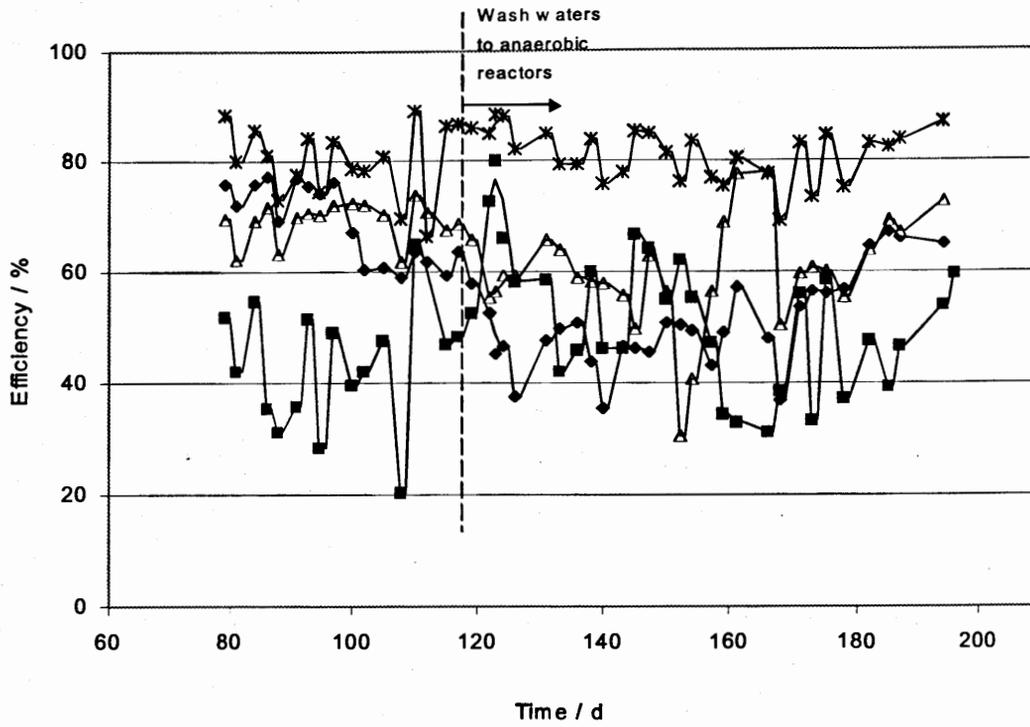
Figure 5: The treatment efficiency by the total COD value (TCOD):  $\blacklozenge$  - anaerobic reactor #1,  $\blacktriangle$  - anaerobic reactor #2,  $\blacksquare$  - anoxic reactor,  $\times$  - the whole system.
