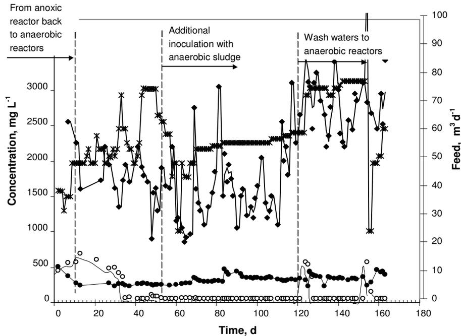
**Figure 9.** Hydraulic loading rate (feed,  $\text{m}^3 \text{d}^{-1}$ ) and the content of sulfates and sulfides ( $\text{mg L}^{-1}$ ) in the effluent from anaerobic reactor 2:  $\blacklozenge$  - sulfates inlet,  $\circ$  - sulfates outlet,  $\bullet$  - sulfides,  $\times$  - feed.
