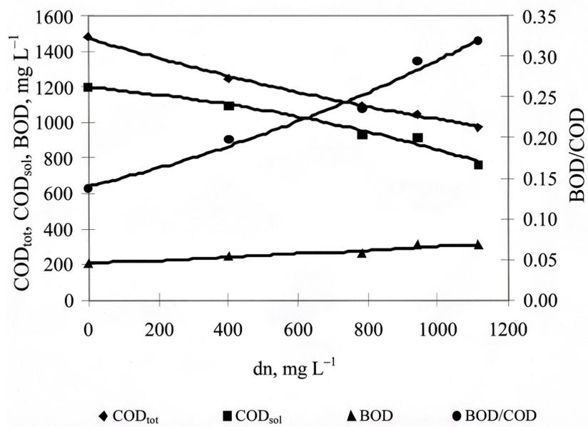
**Figure 17.** The effect of ozone dosage  $dn$  on  $COD_{tot}$ ,  $COD_{sol}$ , BOD, and BOD/COD of biologically treated yeast wastewater (run 3). The pH rose from 7.3 to 7.9.
