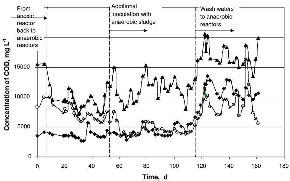
**Figure 11.** Concentration of total chemical oxygen demand (TCOD,  $\text{mg L}^{-1}$ ) in anaerobic reactors: ▲ - TCOD of the inflow to the mixing tank, ◆ - TCOD of reactor 1, ○ - TCOD of reactor 2.
