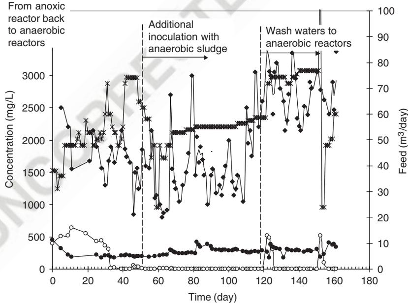
Fig. 3. Hydraulic loading rate (feed, m<sup>3</sup>/day) and the content of sulphates and sulphides (mg/L) in the effluent from anaerobic reactor 2: ♦, sulphates inlet; ○, sulphates outlet; ●, sulphides; ×, feed.
