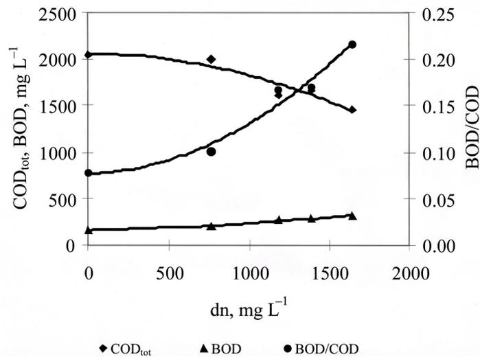
**Figure 15.** The effect of ozone dosage (dn) on COD<sub>tot</sub>, BOD, and the ratio BOD/COD of biologically treated yeast wastewater (run 1). The pH rose from 7.3 to 7.9
