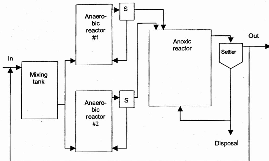
Figure 1: The technological set-up used in the Salutatguse Yeast Factory (Kohila, Estonia) with the recirculation of the outlet flow from the anoxic reactor back to the anaerobic reactors. S- settler.
