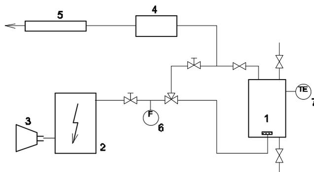
**Figure 6.** Laboratory set-up for batch ozonation. 1 – semi-batch reactor, 2- ozone generator Ozon-2M, 3 – air compressor, 4 – ozone analyzer Anseros GM-6040, 5 – residual ozone destruction unit, 6 – flow meter, 7 - thermometer
