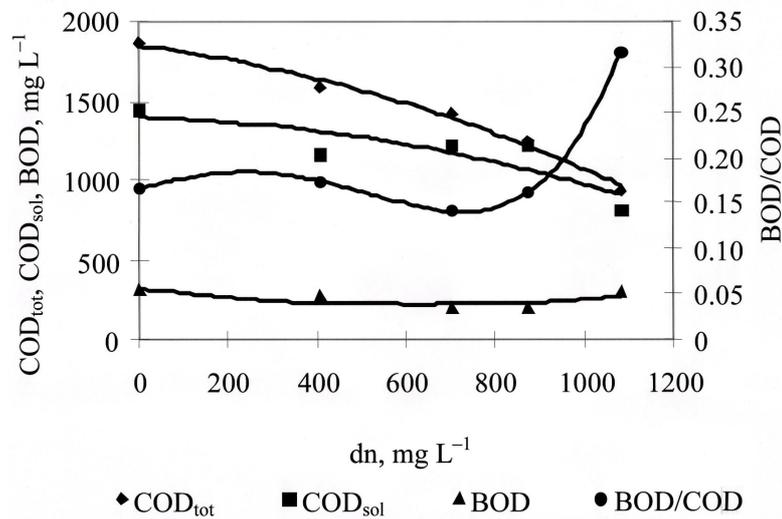
**Figure 18.** The effect of ozone dosage  $dn$  on  $COD_{tot}$ ,  $COD_{sol}$ , BOD, and the ratio BOD/COD of biologically treated yeast wastewater (run 4). The pH rose from 7.3 to 7.9.
