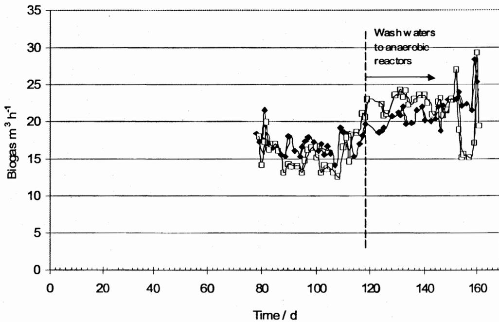
Figure 6: Production of biogas in the anaerobic reactors:  $\blacklozenge$  - reactor #1;  $\square$  - reactor #2.
