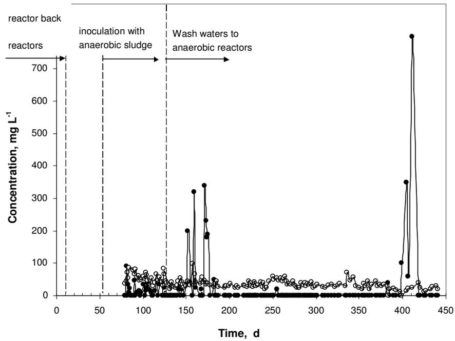
**Figure 10.** Influence of re-circulation on the concentration of sulfates and sulfides in anoxic reactor: ● - sulfates ( $\text{mg L}^{-1}$ ), ○ - sulfides ( $\text{mg L}^{-1}$ )
