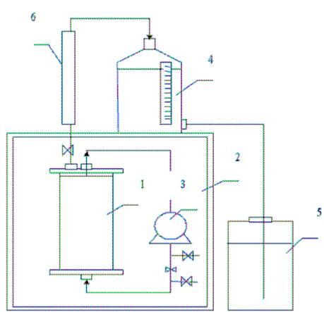
**Figure 4.** Laboratory set-up for anaerobic sequencing batch reactor (ASBR). 1- anaerobic reactor, 2-thermostat, 3-peristaltic pump, 4-wet gas meter, 5-water collector, 6 – alkali lock
