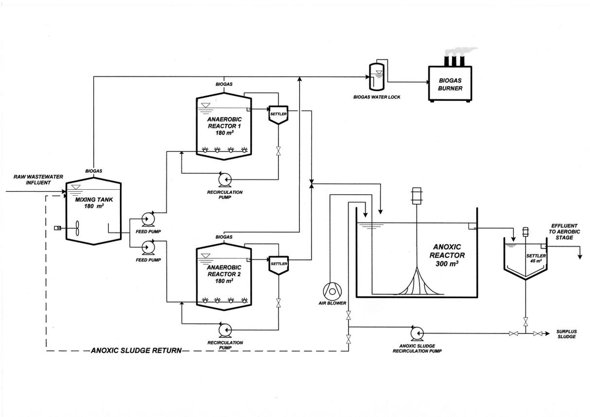
**Figure 7.** The technological set-up used in the Salutagus Yeast Factory with re-circulation of the sludge from anoxic reactor back to the inlet, i.e. to the mixing tank
