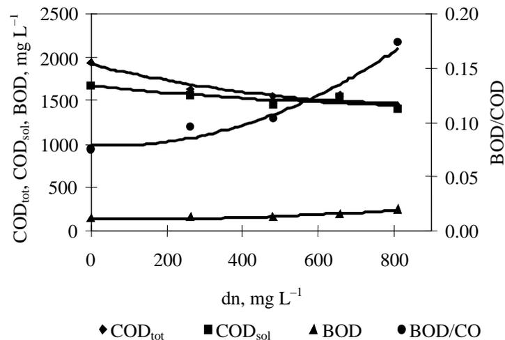
**Fig. 7.** The effect of ozone dosage (dn) on COD<sub>tot</sub>, COD<sub>sol</sub>, BOD, and the ratio BOD/COD of biologically treated yeast wastewater (run 5). The pH rose from 7.9 to 8.4.
