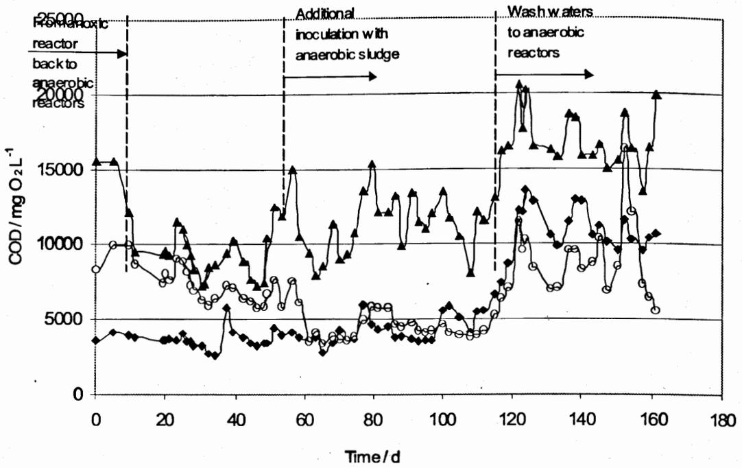
Figure 3: Total chemical oxygen demand (TCOD) values of anaerobic reactors: ▲ - TCOD of the inflow to the mixing tank, ◆ - TCOD of reactor #1, ○ - TCOD of reactor #2.
