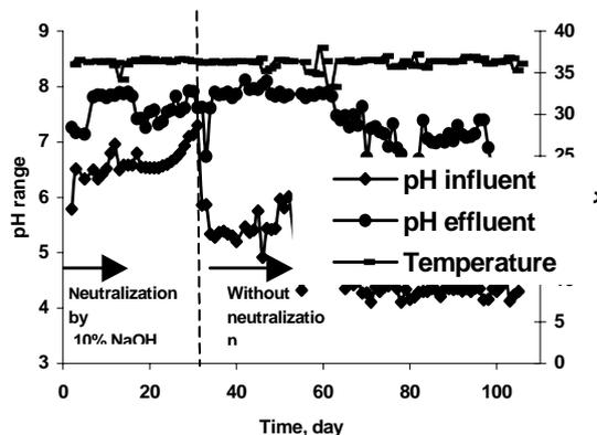
Fig. 3. Temperature and pH changes time
