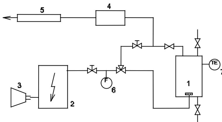
**Fig. 2.** Laboratory set-up for batch ozonation. 1 – semi-batch reactor, 2 – ozone generator Ozon-2M, 3 – air compressor, 4 – ozone analyser Anseros GM-6040, 5 – residual ozone destruction unit, 6 – flow meter, 7 – thermometer.
