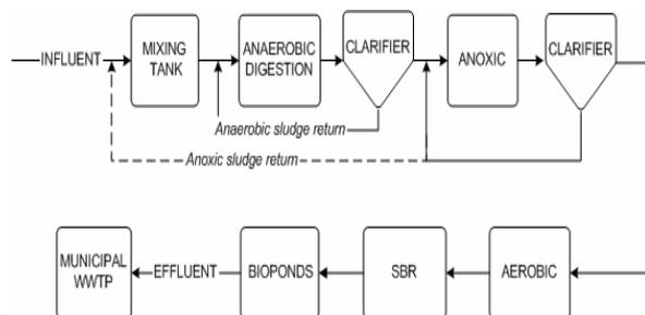
Fig. 4. The principal scheme of wastewater treatment in Yeast Factory (Estonia)
