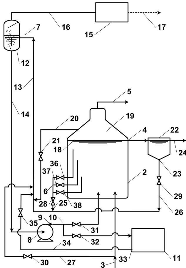
**Figure 20.** Device of anaerobic purification of wastewater with obtaining of biogas.
