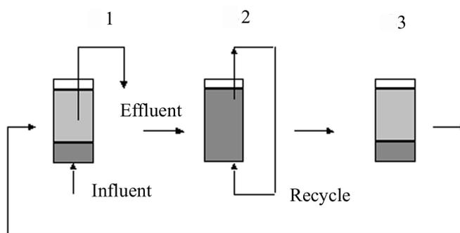
**Fig. 2.** Operation cycles of an ASBR. 1 – filling and decanting cycle, 2 – reaction cycle, 3 – sludge settling.
