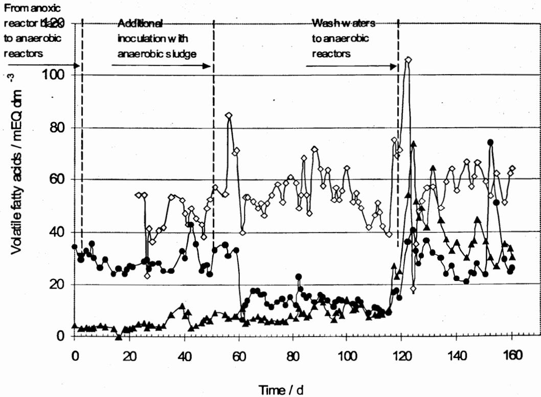
Figure 4: Concentration of volatile fatty acids (VFAs) ◇ - in the mixing tank, ▲ - in the effluent from anaerobic reactor #1, ● - in the effluent from anaerobic reactor #2.
