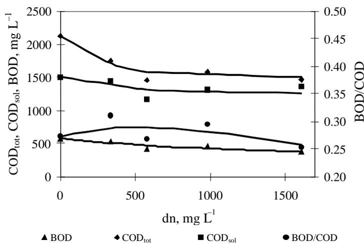
**Fig. 4.** The effect of ozone dosage dn on COD<sub>tot</sub>, COD<sub>sol</sub>, BOD, and BOD/COD of biologically treated yeast wastewater (run 2). The pH fell from 8.3 to 8.1.
