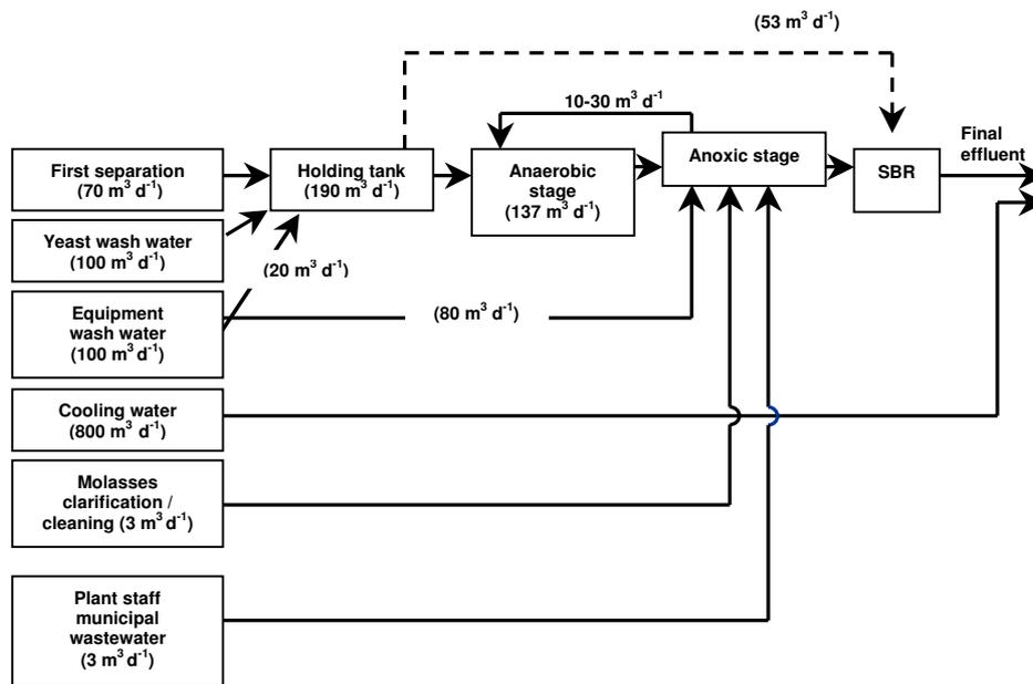
**Figure 8.** Scheme of wastewater streams at Saltaguse Yeast Factory
