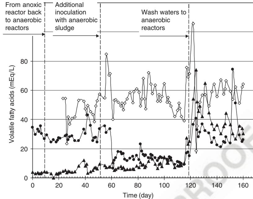
**Fig. 6.** Concentration of volatile fatty acids (mg/L):  $\diamond$ , in the mixing tank;  $\triangle$ , in the effluent from anaerobic reactor 1;  $\bullet$ , in the effluent from anaerobic reactor 2.
