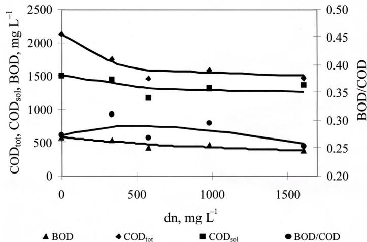
**Figure 16.** The effect of ozone dosage dn on COD<sub>tot</sub>, COD<sub>sol</sub>, BOD, and BOD/COD of biologically treated yeast wastewater (run 2). The pH fell from 8.3 to 8.1
