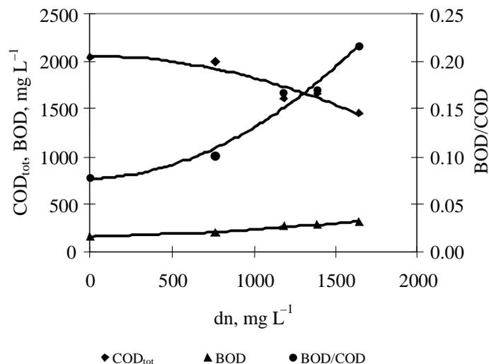
**Fig. 3.** The effect of ozone dosage (dn) on COD<sub>tot</sub>, BOD, and the ratio BOD/COD of biologically treated yeast wastewater (run 1). The pH rose from 7.3 to 7.9.
