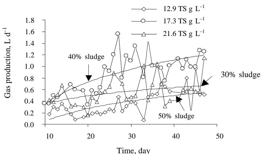
**Fig. 4.** Gas production at different seed sludge contents.
