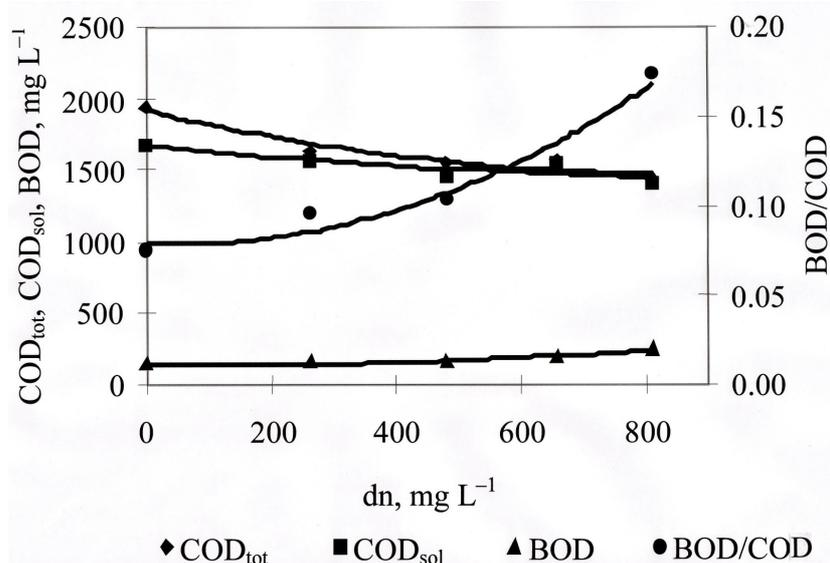
**Figure 19.** The effect of ozone dosage (dn) on COD<sub>tot</sub>, COD<sub>sol</sub>, BOD, and the ratio BOD/COD of biologically treated yeast wastewater (run 5). The pH rose from 7.9 to 8.4.
