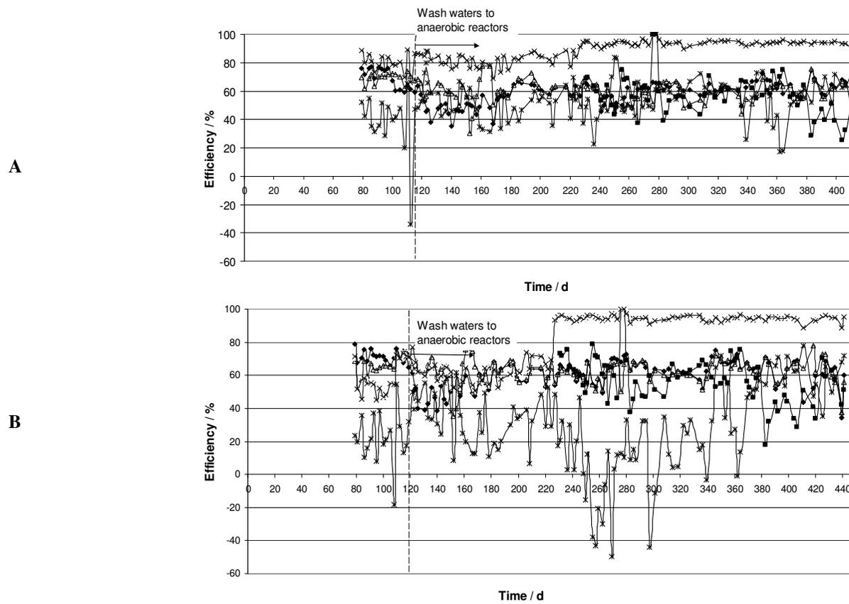
**Figure 13.** The treatment efficiency: **A**) by the total COD value (TCOD, %), **B**) by the soluble COD value (SCOD, %). ◆ - anaerobic reactor 1, △ - anaerobic reactor 2, \* - anoxic reactor, - sequenced batch reactor, × - the whole system.
