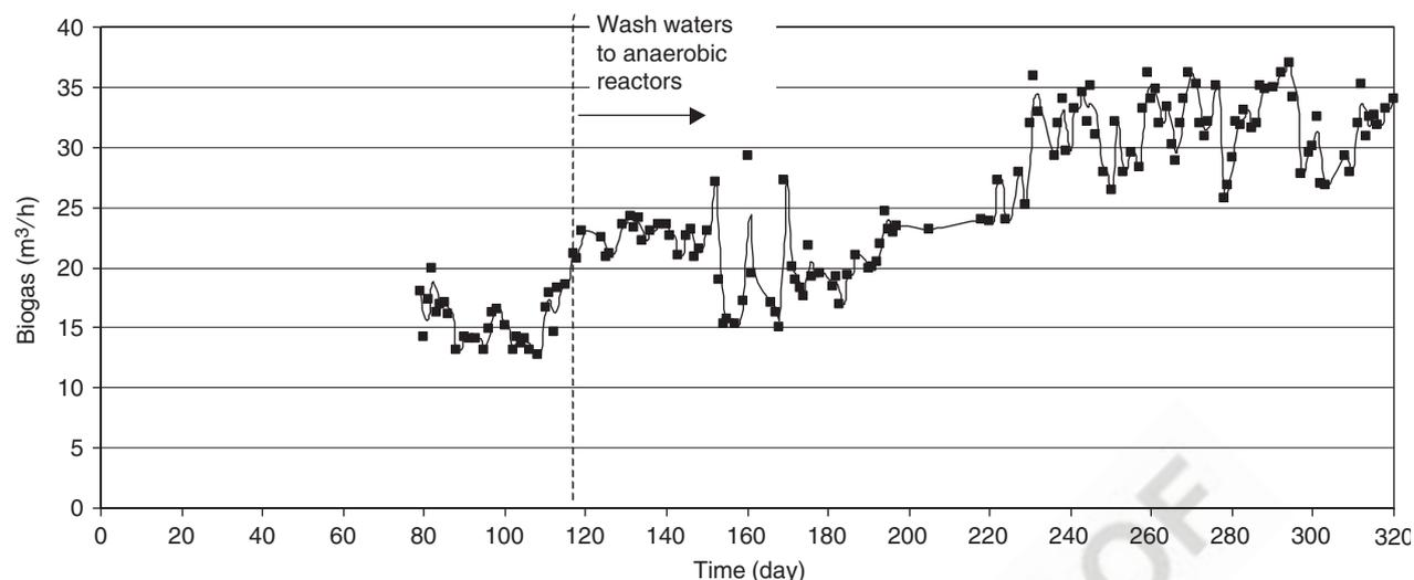
Fig. 8. Production of biogas in the anaerobic reactor 2 ( $\text{m}^3/\text{h}$ ).
