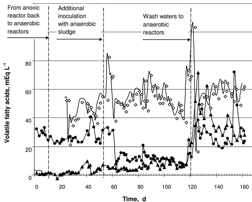
**Figure 12.** Concentration of volatile fatty acids (VFAs, mg L<sup>-1</sup>): ◇ - in the mixing tank, ▲- in the effluent from anaerobic reactor 1, ●- in the effluent from anaerobic reactor 2.
