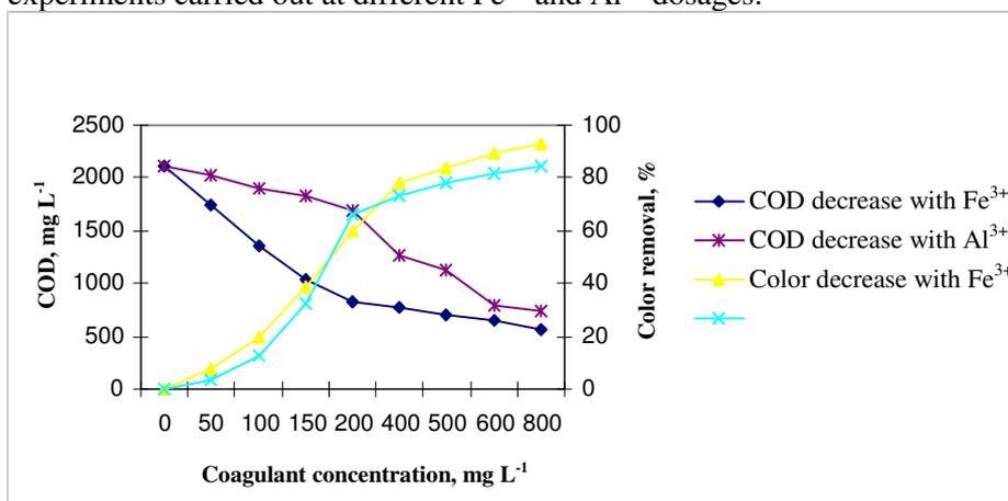
**Figure 14.** Effect of Fe<sup>3+</sup> and Al<sup>3+</sup> dosages on color and COD removal during coagulation experiments
