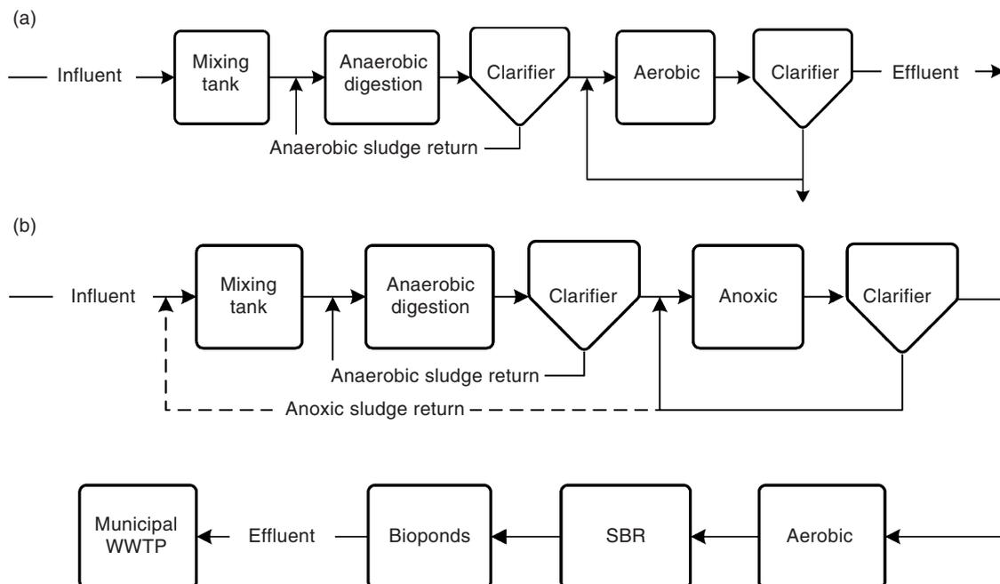
**Fig. 1.** (a) The original treatment facility of OY Tampella Ab (Finland); (b) the technological set-up used in the Salutaguse Yeast Factory with recirculation of the effluent from anoxic reactor back to the inlet. SBR, sequencing batch reactor; WWTP, wastewater treatment plant.
