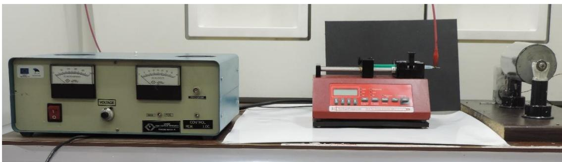
Figure 14. Electrospinning apparatus
