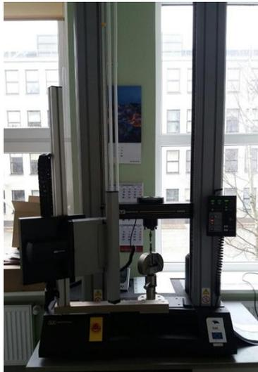
Figure 16. Tensile testing machine Instron 5866
