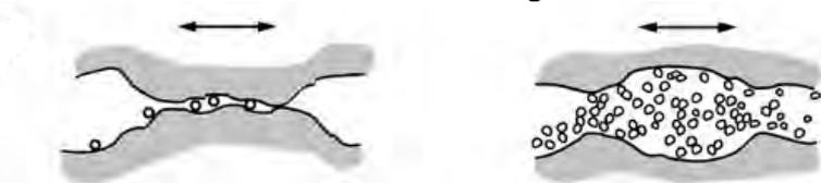
**Figure 1.32.** The basic mechanism of chemical wear [90].
