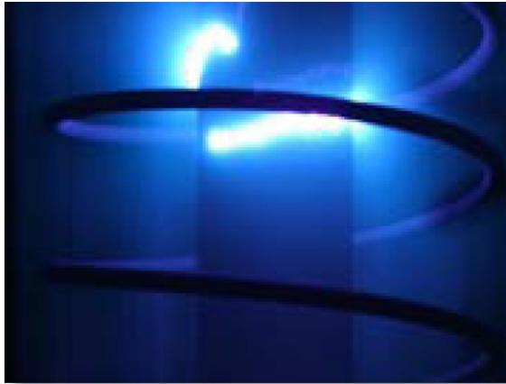
**Figure 1.13.** Photograph of the vacuum arc, rotating around the cathode due to the axial magnetic field generated by the helical solenoid [61].
