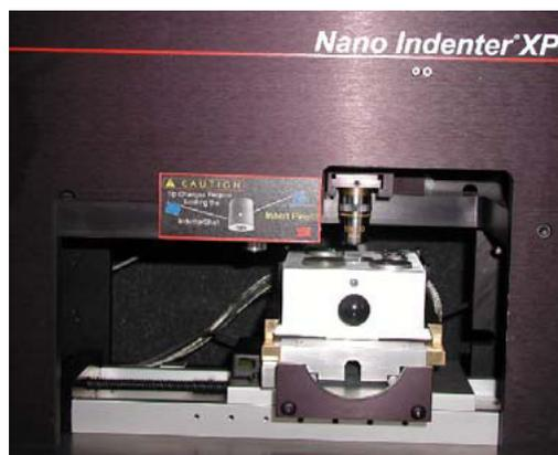
**Figure 2.4.** The nanoindentation platform that was used to evaluate nanohardness of selected PVD coatings at Uppsala University.
