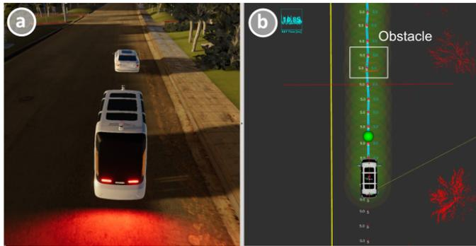
Figure 21: a) The LGSVL simulator simulates an overtaking scenario. b) A ROS visualization shows vehicle sensors, waypoints, and position on a map. Figure from article V.
