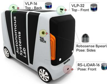
Fig. 2. Ego digital twin; 3D model with the sensor configuration
