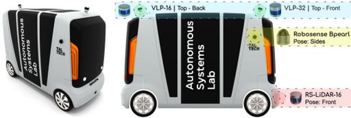
**FIGURE 12** The iseAuto shuttle bus with the indication of the position of its three different types of Lidars
