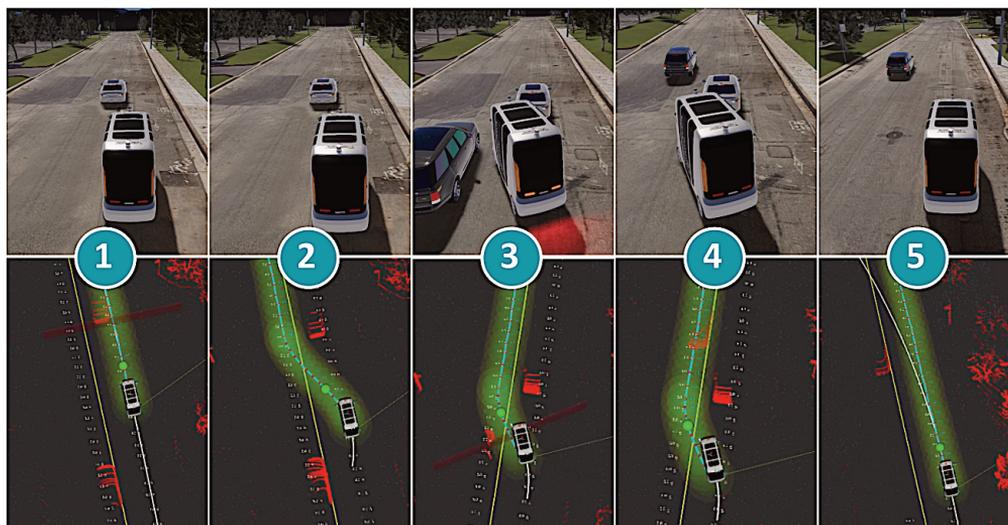
Fig. 10. Different steps of an overtaking process.
