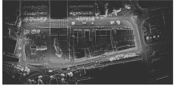
Fig. 5. A Point cloud map is created based on Lidar data.
