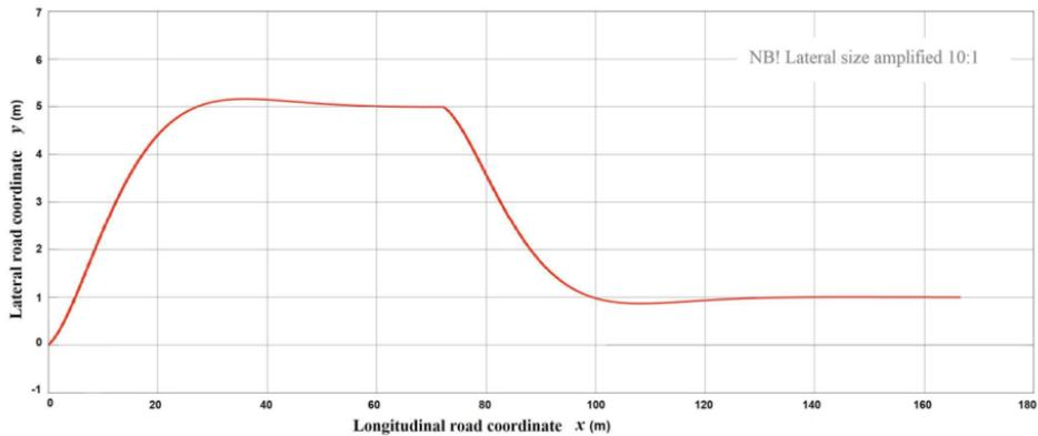
Figure 26: A calculated trajectory consists of two steps: a left shift of 5 m from the initial lane  $y = 0$ , followed by a right shift of 1 m back to its original lane  $y = 0$ . Figure from article VI.
