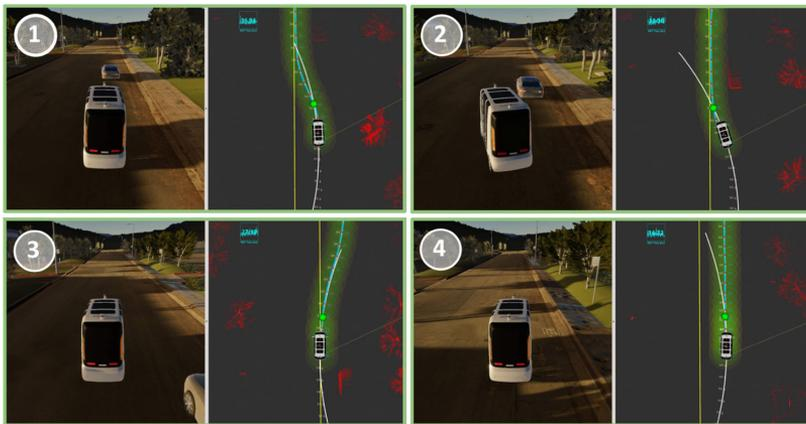
**FIGURE 10** Four characteristic time instants in SVL and the corresponding ROS simulation environment, describing the overtaking maneuver based on the smooth sigmoid-based path
