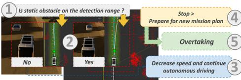
FIGURE 5 Five decision-making steps of the overtaking algorithm in the case an obstacle was detected by the shuttle
