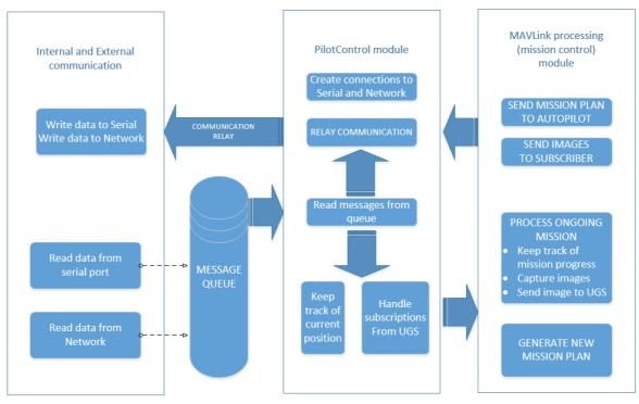
Figure 17: Pilot Control module
