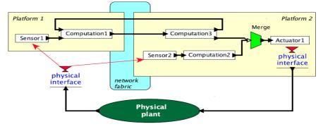
Figure 8: Structure of a cyber-physical system [22]
