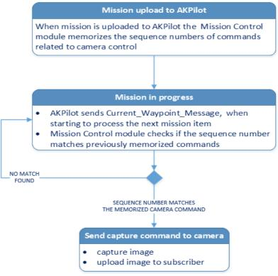
Figure 19: Camera control procedure
