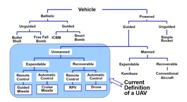
Figure 2: UAV family tree [2] (RPV – Remotely piloted vehicle, ICBM – Inter Continental Ballistic Missile)
