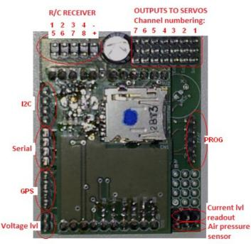
Figure 13: AKpilot connections
