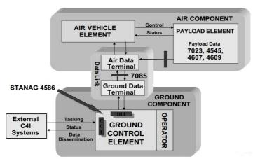
Figure 3: STANAG for UAV control [8]
