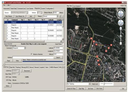
Figure 22: Generated mission plan downloaded from AKPilot
