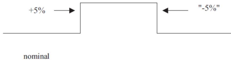
Figure 3.2 Application of test signal
