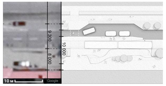
Figure 7-7: Layout for limited space with one-way traffic
