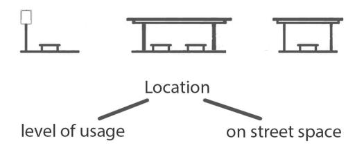
Figure 2-3: Primary design factors for a bus stop
