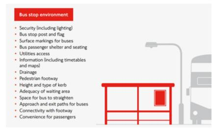
Figure 2-4: Features of the bus stop environment [7]
