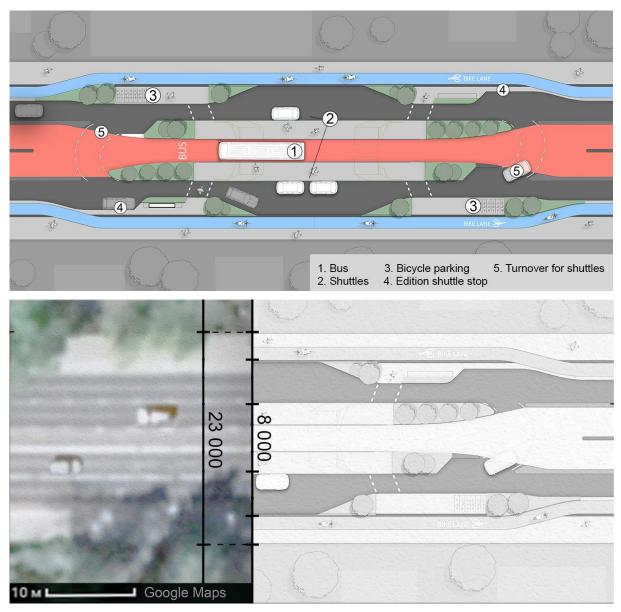
Figure 7-8: Layout for limited space street with two-way direction
