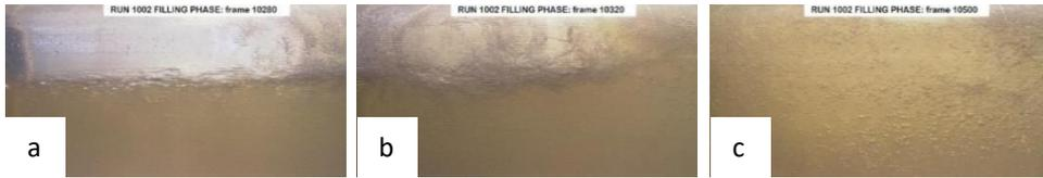
Figure 25. (a) Stratified, (b) roller and (c) bubbly flow stages of pressurisation bore advancement in a 235 mm pipe with comparatively larger filling ratio (Laanearu & van't Westende, 2010). The filling ratio upstream of the hydraulic jump is 0.53 (frame a).
