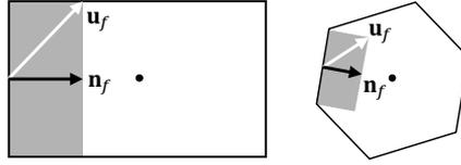
Figure 9. The face normal of a cell is oriented towards the cell centre.
