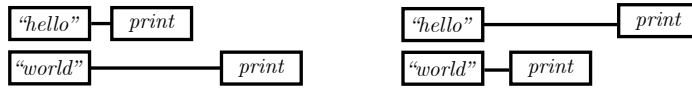
Figure 2.6: These string diagrams are no longer equal in an effectful category. This makes effectful categories suitable for the semantics of programming languages, where the order of effectful processes (such as printing) matters.
