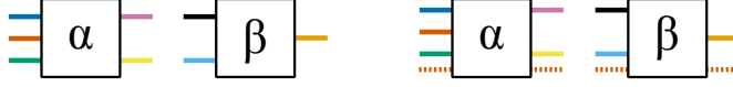
Figure 3.23: Left: A monoidal graph \mathcal{G} . Right: the associated runtime monoidal graph \mathcal{G}_R , where the new sort R is drawn as a dashed string.
