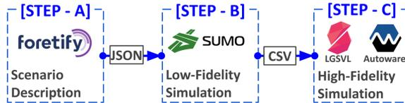
Figure 3.14: Three main steps of the two-layer validation method. The data format transferred between the layers is annotated.
