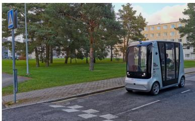
**FIGURE 1.** TalTech iseAuto - an AV shuttle.
