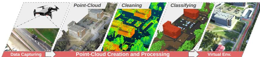
Figure 2.7: Steps to build a virtual environment from aerial imagery
