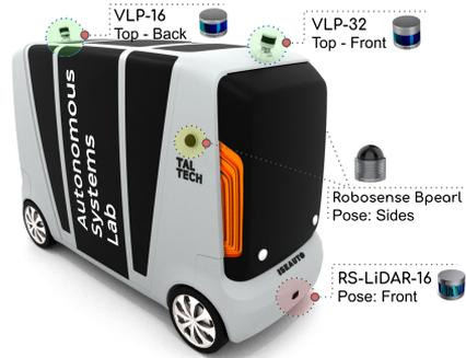
FIGURE 7. iseAuto simulated model with different LiDARs installed.
