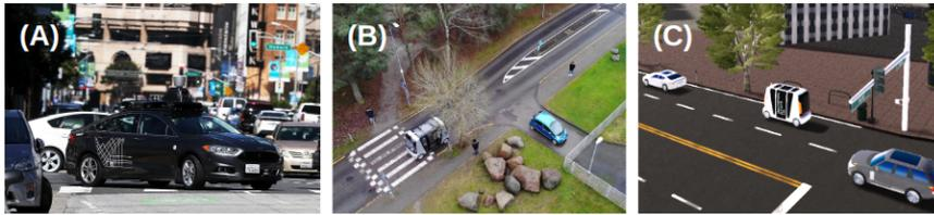
Figure 1.3: Three main AV testing platforms: a) On-road testing b) Track testing c) Simulation
