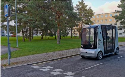
Figure 1: iseAuto autonomous shuttle
