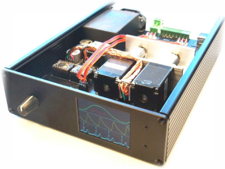
Fig. 11. Emulator of the cardio-respiratory dynamic impedance [22].
