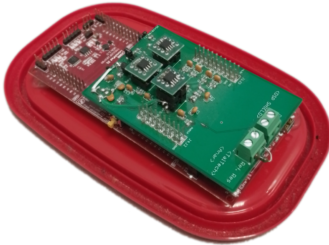
Figure 3: Photo of the first-generation DSP-based impedance measurement prototype, developed during this PhD work.
