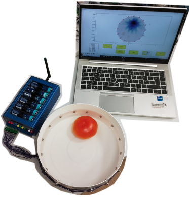
Fig. 1. Experimental setup of the DSP-based EIT system
