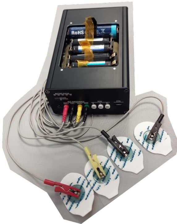
Figure 5: Photo of the second-generation DSP-based EBI, ECG, and PPG device
