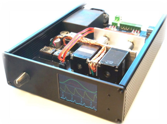
Fig. 3. Emulator of the cardio-respiratory dynamic impedance [13]
