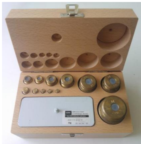
Figure 4.2. Weights used at the adjustment of the load cell
