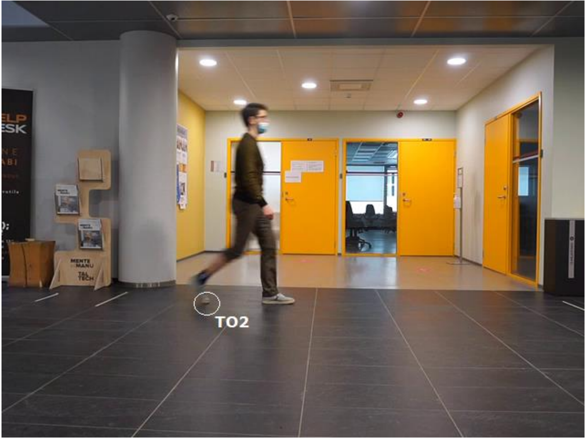
Figure 4.2 An example of the toe-off event of the right leg extracted from the video recordings. The results of the video labeling are summarized in the table given in APPENDIX 1. Based on the results, with equation (3.1), stride durations were calculated. The summary of these calculations is presented in Table 4.1.
