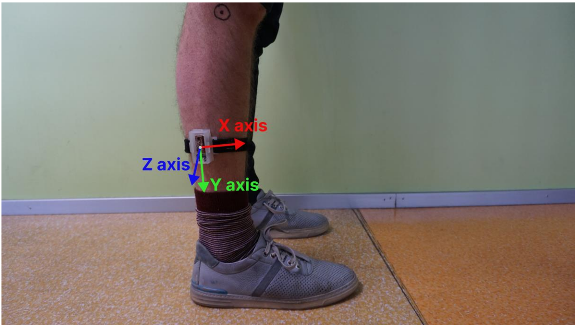
Figure 3.11 Sensor attached to the shank with arrows representing axes of the accelerometer
