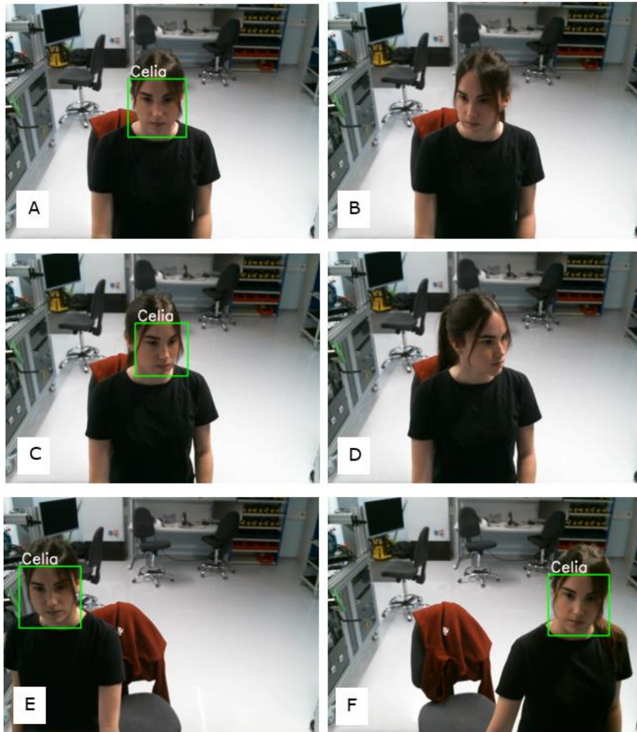
Figure 4.19 Face recognition in user's different appearance A, B, C, D - user's head rotations; E, D - user's position in the edges of the frame
