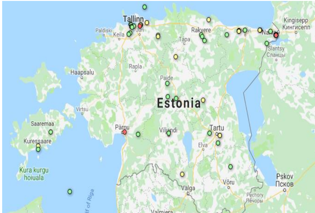
Figure 4 Estonian thermal power plants and CHP plants. Colors-separated power: Green - 0... 1.9 MW; yellow - 1.9 to 20 MW; red - 20... 195 MW source: energiatalgud.ee
