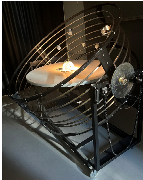
Figure 6 Heliodon. Tallinn University of Technology
