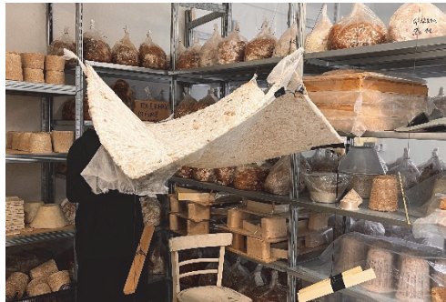
Figure 3 Forming of the mycelium on gravity-shaped fabric form
