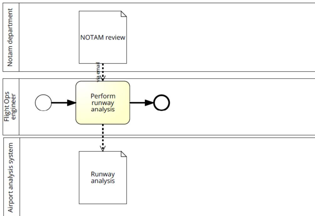
Figure 35. Runway analysis subprocess, expanded. (Rein Nõukas)
