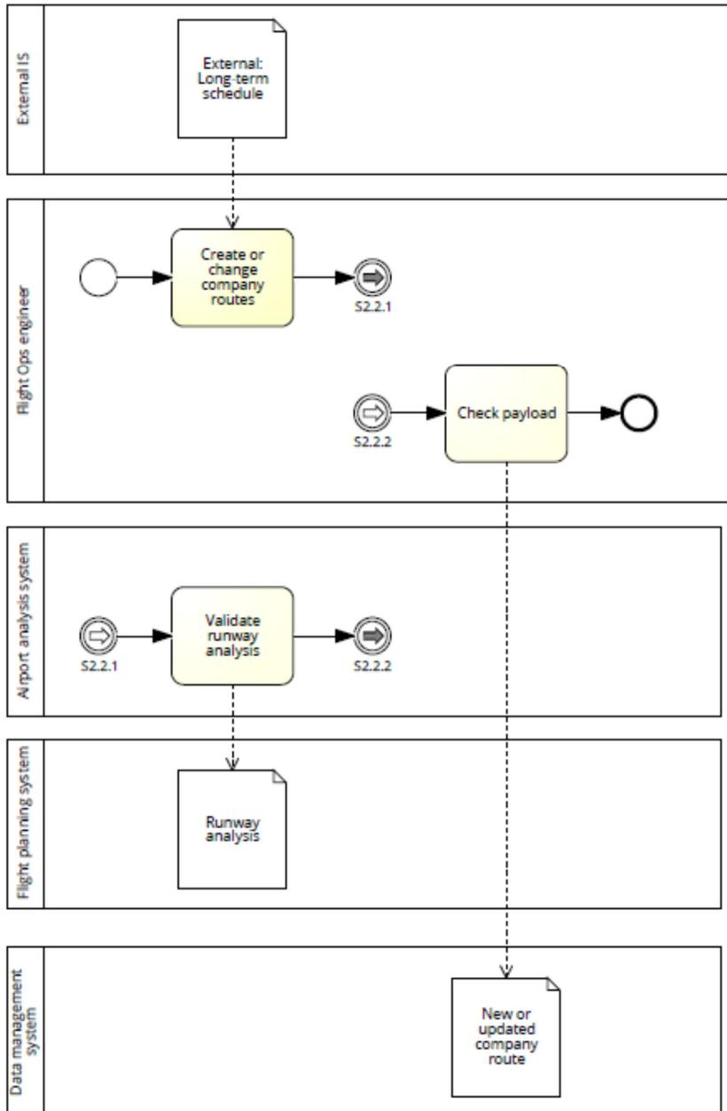
Figure 18. Company routes management subprocess, expanded. (Rein Nõukas)
