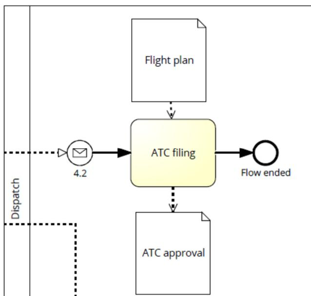
Figure 40. ATC filing workflow. (Rein Nõukas)
