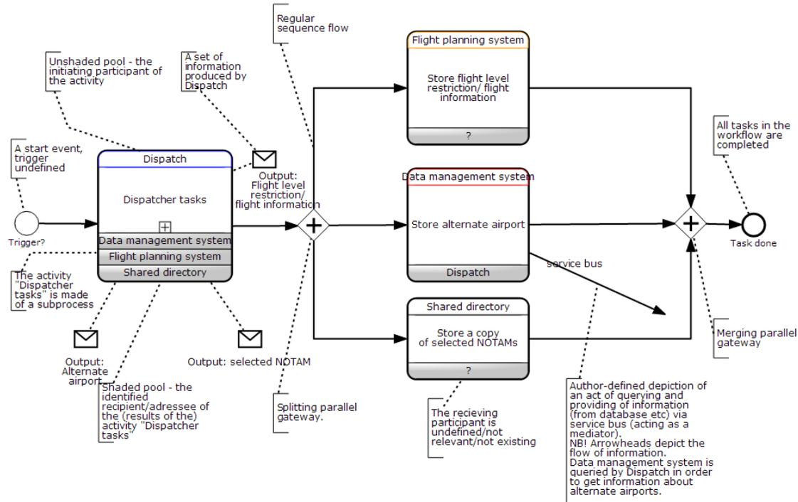
Figure 6. Dispatcher operation subprocess. (Rein Nõukas)
