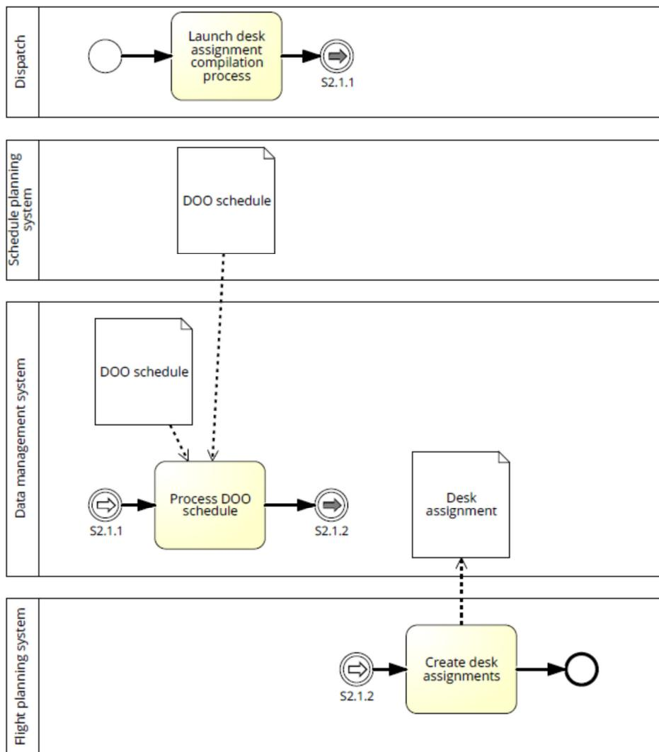
Figure 24. Desk assignment compilation subprocess, expanded. (Rein Nõukas)
