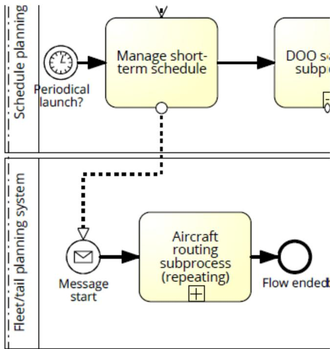
Figure 10. Aircraft routing workflow. (Rein Nõukas)
