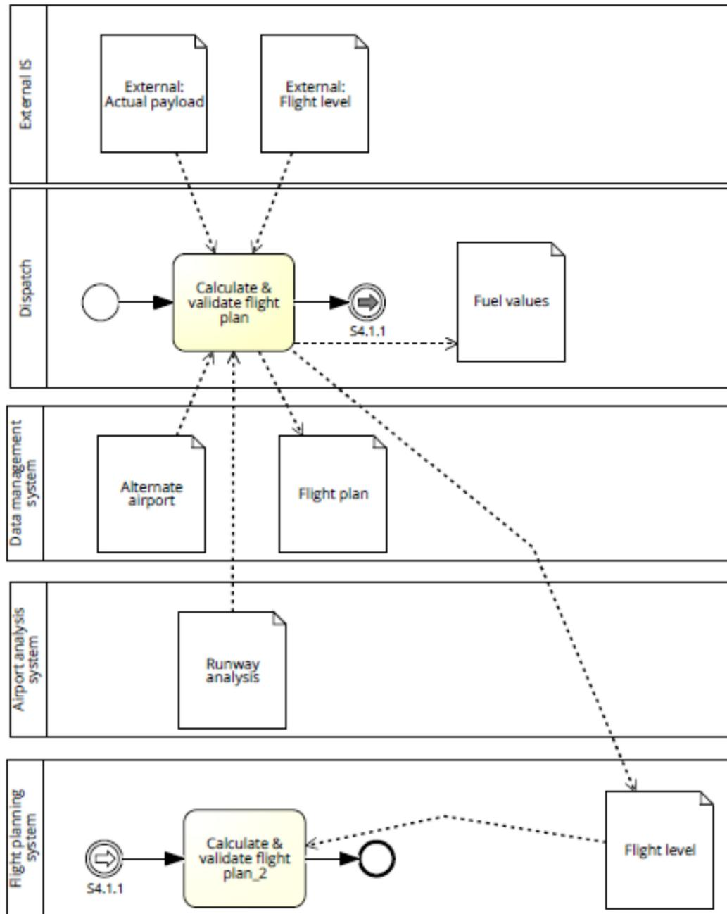
Figure 37. Flight plan calculation & validation subprocess, expanded. (Rein Nõukas)
