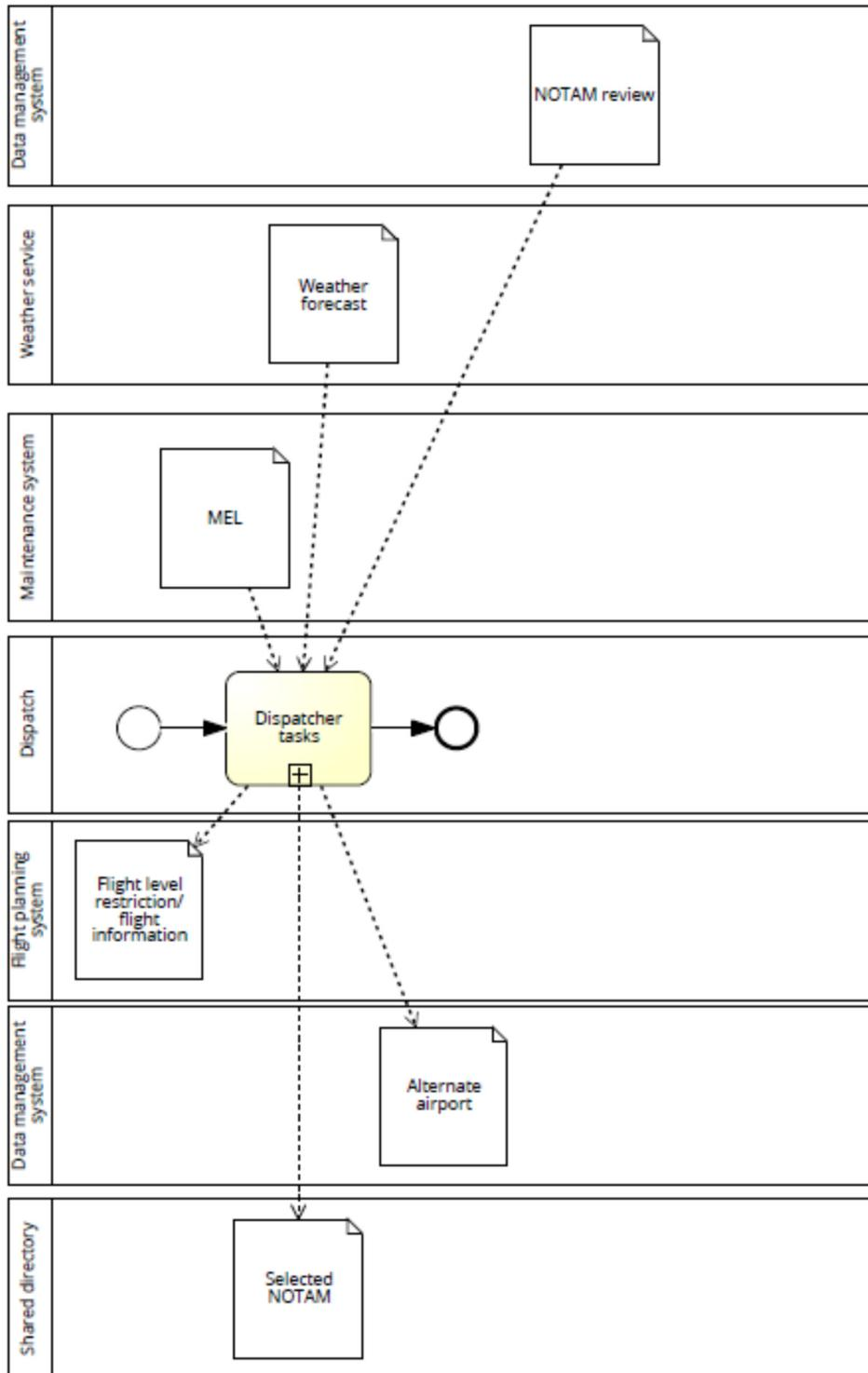
Figure 32. Dispatcher operations subprocess, expanded. (Rein Nõukas)
