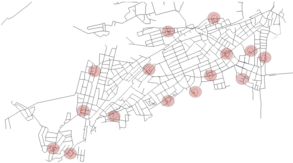
Figure 2-11 Pumping stations in Area 4 [Adapted from Puust et al. (2014)]
