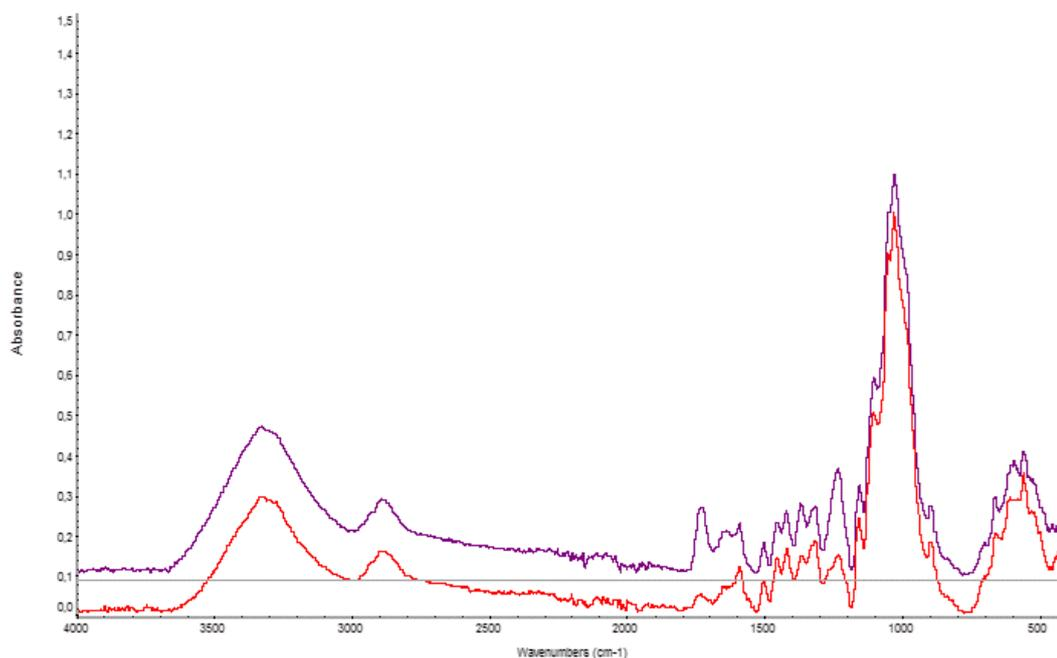
**Figure 3.1.** The IR spectra of aspen wood (violet) and BCTMP (red).
