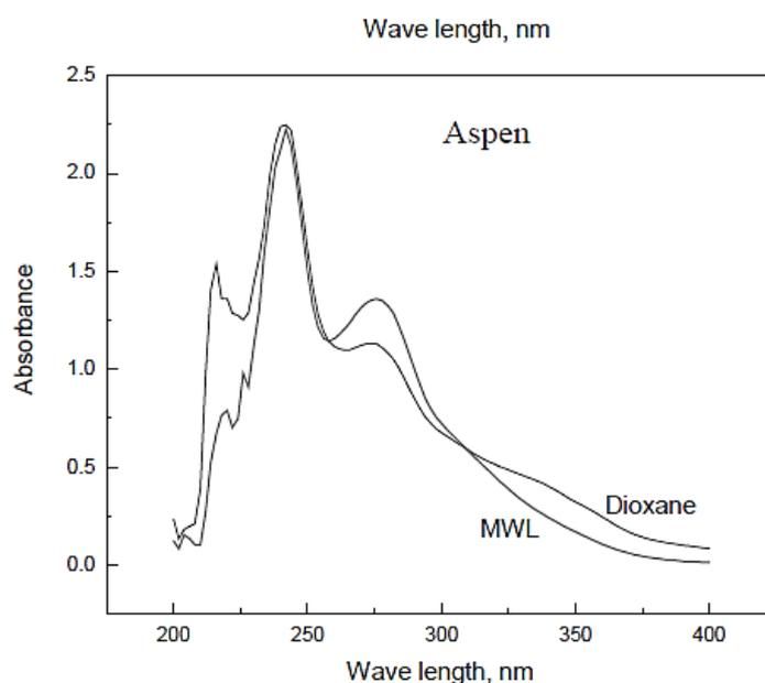
**Figure 1.14.** UV spectra of MWL and dioxane lignin from Aspen (Jahan & Mun 2010).
