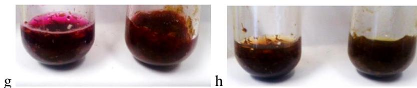
**Figure 3.11.** Photos show suspension of aspen wood (left) and BCTMP (right) samples treated with 1%  $\text{KMnO}_4$  solution for 2 minutes (g) and 10 minutes (h)
