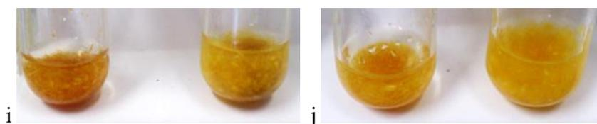
**Figure 3.12** Photos show suspension of aspen wood (left) and BCTMP (right) samples treated with 3 % HCl solution for 20 s (a) and 2 minutes (b).
