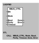
*Fig. 21 Exchange initialization block.*
