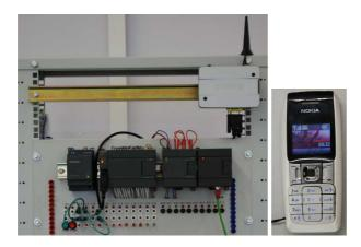
Fig. 16 Set-up with a GSM modem.
