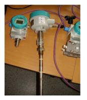
Fig. 3.14 Pointek CLS 300 level switch.
