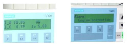
Fig. 14 Current parameters and alarm signals of the Text Display TD200.
