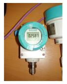
Fig. 3.12 SITRANS P DS III transmitter.
