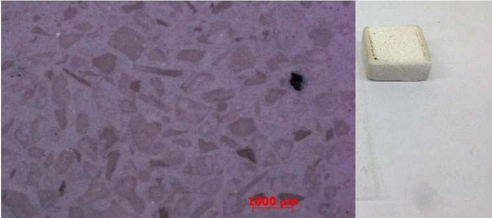
Figure 30. Specimen No.1 after test at 600 °C , commercial ceramics Rescor 750 based on SiO<sub>2</sub>
