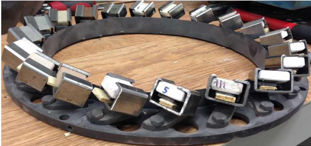
Figure 27. Fixed specimens on the rim of rotor for test at room temperature
