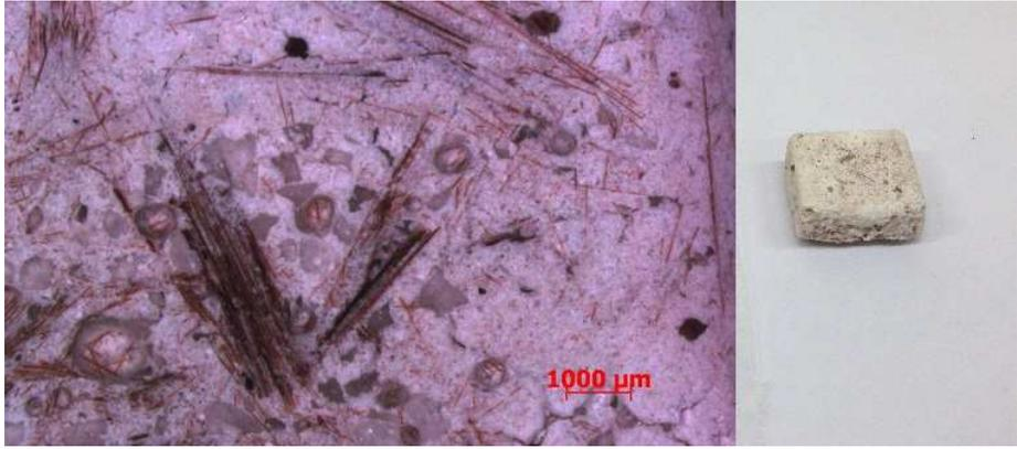
Figure 35. Specimen No.6 after test at 600 °C, commercial ceramics Rescor 750 reinforced with 11wt.% of basalt fiber. Bundles of basalt fiber are visible
