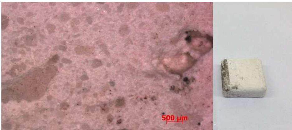
Figure 42. Specimen No.13 after test at 600 °C, commercial ceramics Rescor 780 (based on alumina oxide)
