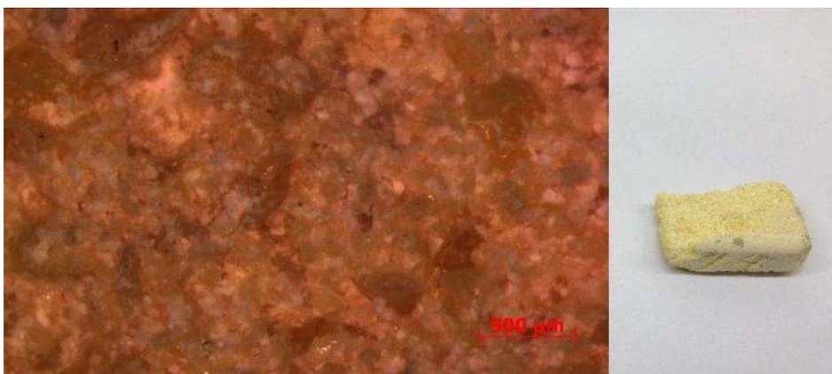
Figure 43. Specimen No.14 after test at 600 °C, commercial ceramics Rescor 780 (based on zirconium oxide)
