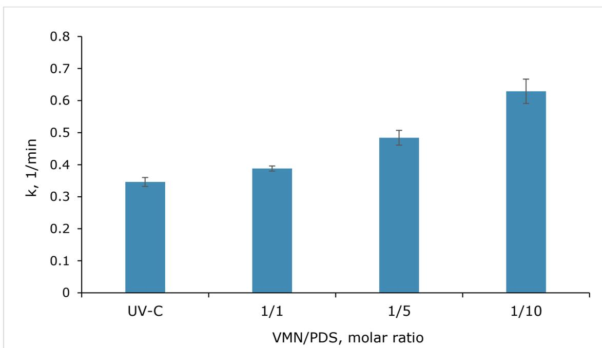
Figure 11. VMN decomposition rate constants by the UV-C photolysis and UV-C/PDS process at different VMN/PDS molar ratios ( $[VMN]_0=13.4 \mu M$ , pH initial)
