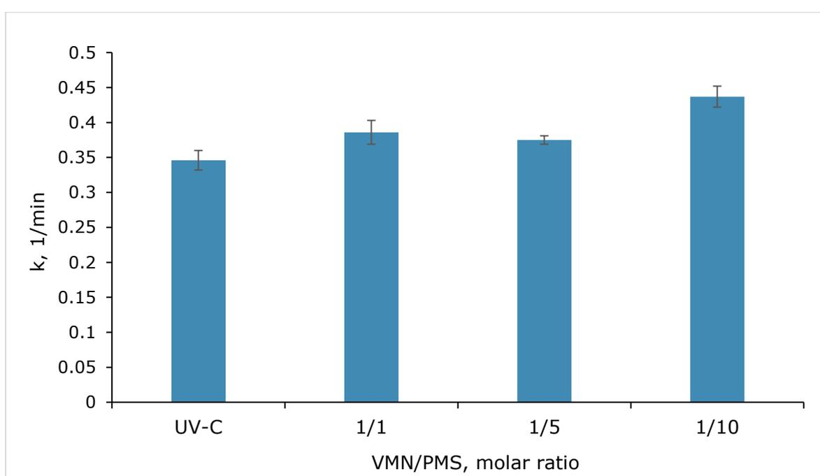
Figure 9. VMN decomposition rate constants by the UV-C photolysis and UV-C/PMS process at different VMN/PMS molar ratios ( $[\text{VMN}]_0=13.4 \mu\text{M}$ , pH initial)
