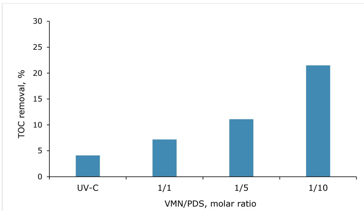
Figure 12. TOC removal by the UV-C photolysis and UV-C/PDS process at different VMN/PDS molar ratios ( $[VMN]_0=13.4 \mu M$ , pH initial,  $t=180$  min)
