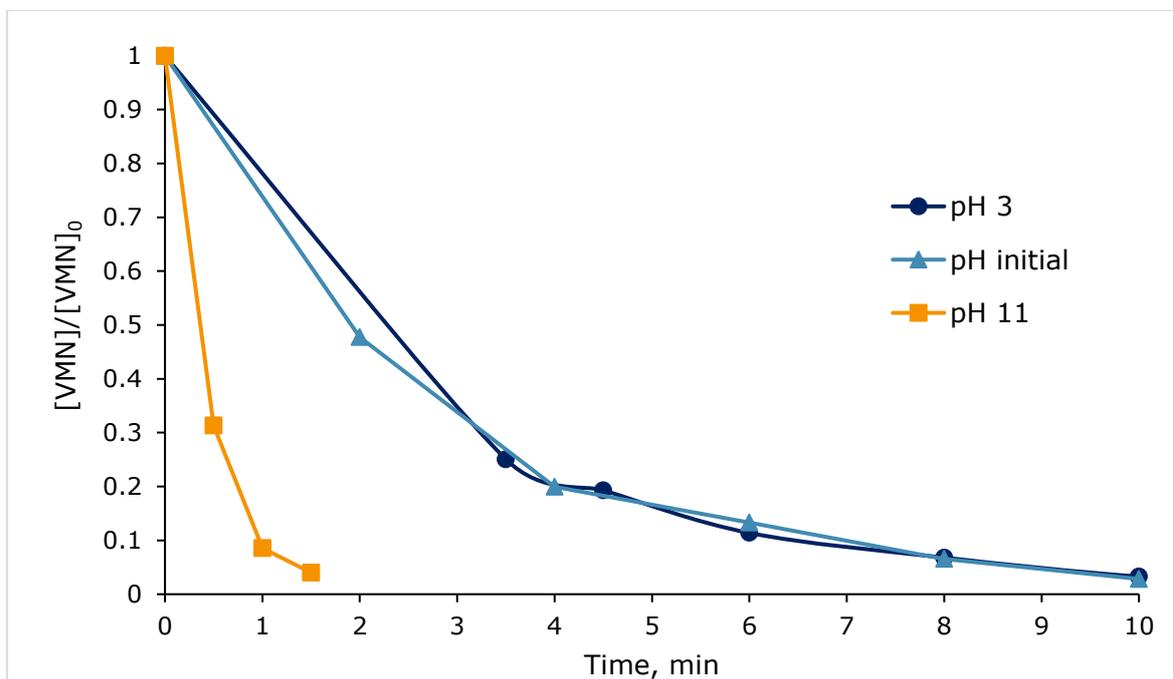
Figure 6. VMN decomposition by the UV-C photolysis at different pH values ( $[VMN]_0=13.4 \mu M$ )
