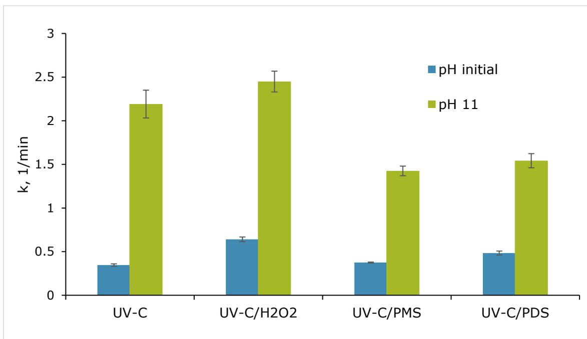
Figure 13. VMN decomposition rate constants by the UV-C photolysis, UV-C/H<sub>2</sub>O<sub>2</sub>, UV-C/PMS and UV-C/PDS processes ([VMN]<sub>0</sub>=13.4 μM, [H<sub>2</sub>O<sub>2</sub>]<sub>0</sub>=[PMS]<sub>0</sub>=[PDS]<sub>0</sub>=67 μM)
