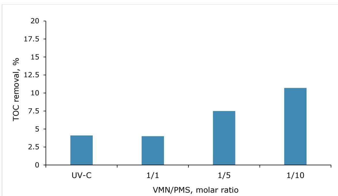
Figure 10. TOC removal by the UV-C photolysis and UV-C/PMS process at different VMN/PMS molar ratios ( $[\text{VMN}]_0 = 13.4 \mu\text{M}$ , pH initial,  $t = 180 \text{ min}$ )
