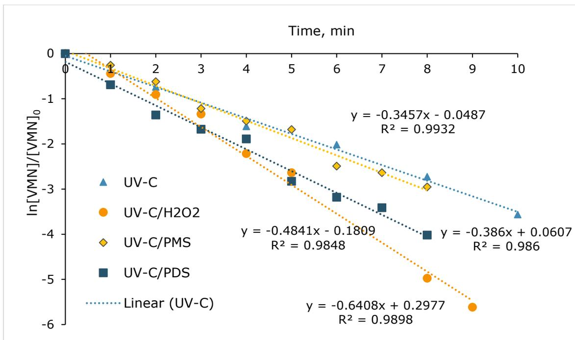
Figure 5. VMN decomposition by the UV-C photolysis, UV-C/H<sub>2</sub>O<sub>2</sub>, UV-C/PMS and UV-C/PDS processes: k values calculation through linear regression ([VMN]<sub>0</sub>=13.4 μM, [H<sub>2</sub>O<sub>2</sub>]<sub>0</sub>=[PMS]<sub>0</sub>=[PDS]<sub>0</sub>=67 μM, pH initial)
