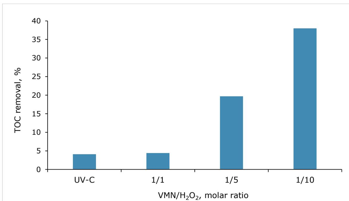
Figure 8. TOC removal by the UV-C photolysis and UV-C/H<sub>2</sub>O<sub>2</sub> process at different VMN/H<sub>2</sub>O<sub>2</sub> molar ratios ( $[VMN]_0=13.4$   $\mu$ M, pH initial,  $t=180$  min)
