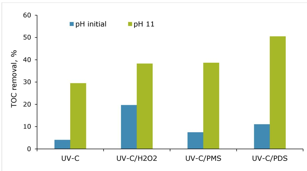
Figure 14. TOC removal by the UV-C photolysis, UV-C/H<sub>2</sub>O<sub>2</sub>, UV-C/PMS and UV-C/PDS processes ([VMN]<sub>0</sub>=13.4 μM, [H<sub>2</sub>O<sub>2</sub>]<sub>0</sub>=[PMS]<sub>0</sub>=[PDS]<sub>0</sub>=67 μM, t=180 min)
