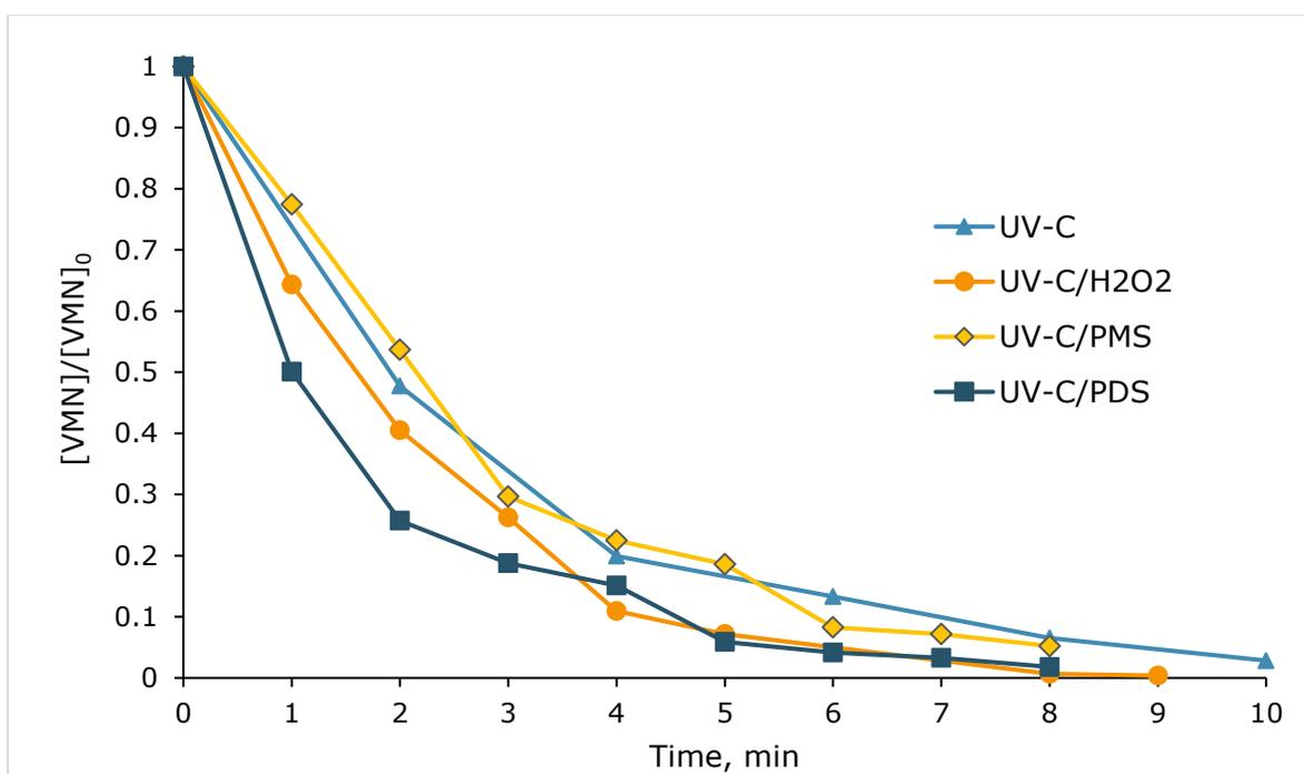
Figure 4. VMN decomposition by the UV-C photolysis, UV-C/H<sub>2</sub>O<sub>2</sub>, UV-C/PMS and UV-C/PDS processes ([VMN]<sub>0</sub>=13.4 μM, [H<sub>2</sub>O<sub>2</sub>]<sub>0</sub>=[PMS]<sub>0</sub>=[PDS]<sub>0</sub>=67 μM, pH initial)
