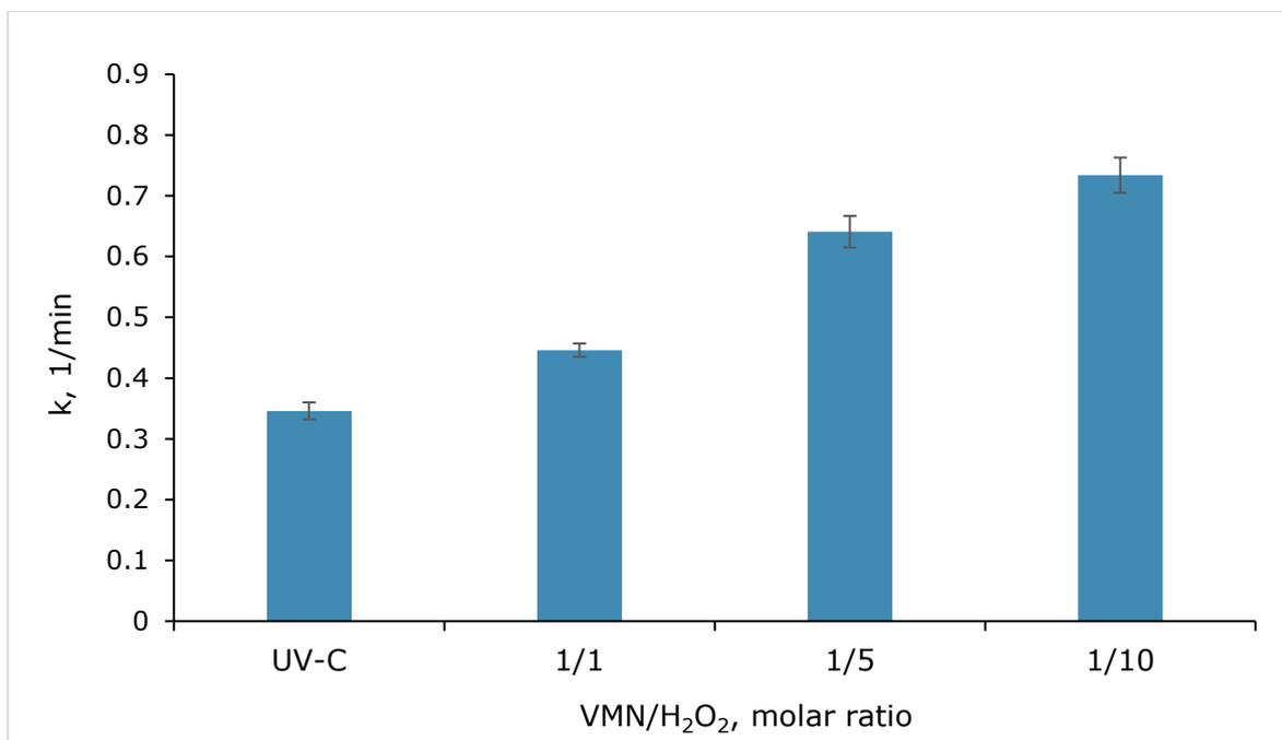
Figure 7. VMN decomposition rate constants by the UV-C photolysis and UV-C/H<sub>2</sub>O<sub>2</sub> process at different VMN/H<sub>2</sub>O<sub>2</sub> molar ratios ([VMN]<sub>0</sub>=13.4 μM, pH initial)
