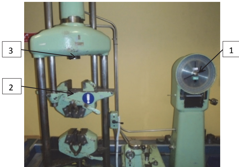
Figure 4.1. Experimental setup: 1- force dynamometer, 2 – fixed table 3 – pressure shaft.
