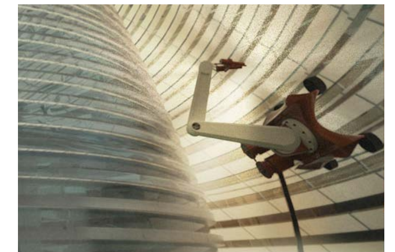
Figure 18. Concept of ice 3D printing robot in Mars Ice House (Montes, 2016)
