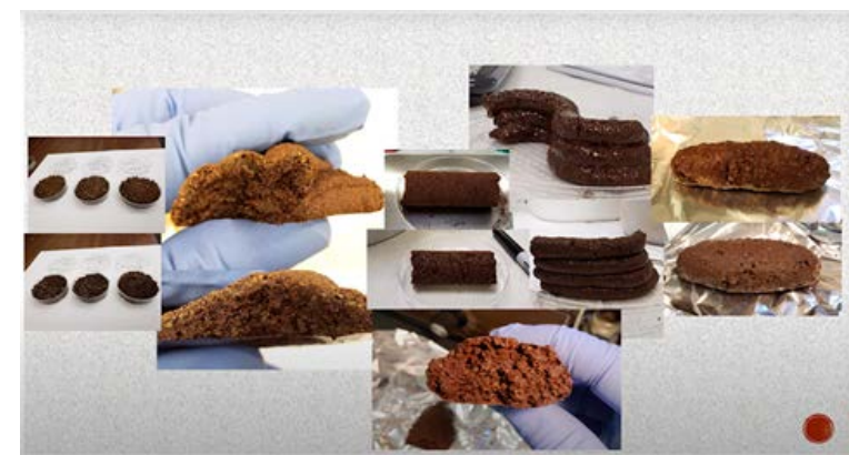
Figure 13. 3D-printing tests with regolith (NASA)
