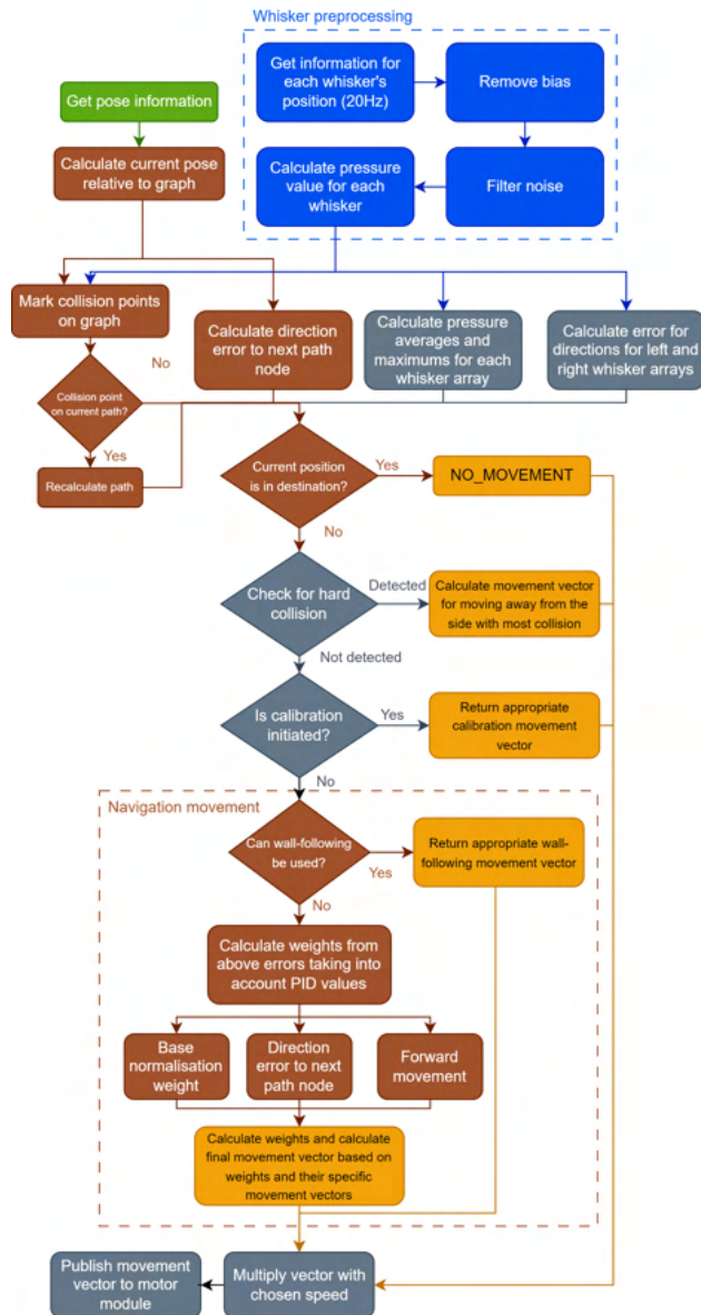
Figure 13. High-level working principle for navigation.
