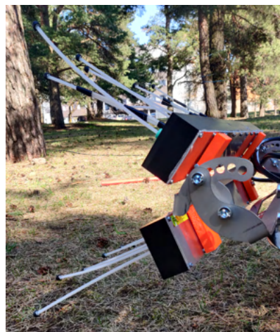
Figure 36. Method of attaching whiskers at an angle.
