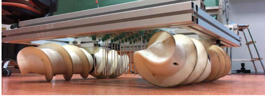
Figure 6. Whisker configuration for ground-based SLAM [7].
