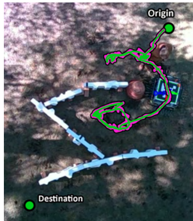
Figure 47. Failed real-world traversal with Theta* due to local loop in utilising wall-following.
