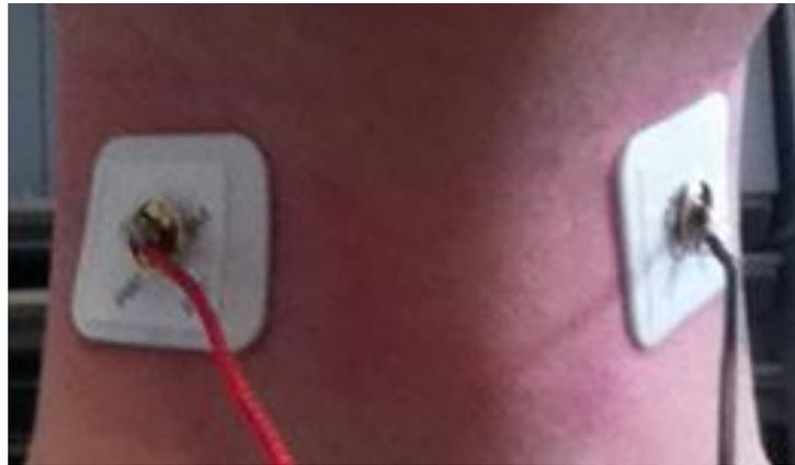
*Figure 26. 3M electrodes in configuration A (horizontal 2 electrode).*
