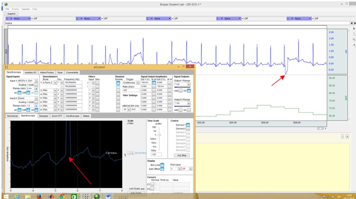
Figure 29. Impedance signal (below) and EKG signal (up) correlation. Artifact is marked with red arrow. 150 kHz signal, configuration E was used.
