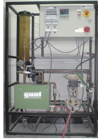
Fig. 11. Level control process (GUNT-RT512) [72].
