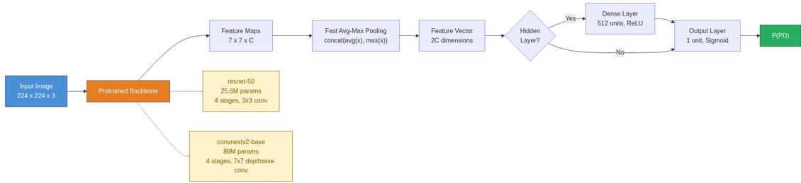
Figure 3. Model architecture for binary PD classification. Both ResNet-50 and ConvNeXtV2-Base share the same classification head: fast average-maximum pooling, an optional hidden layer, and a sigmoid output.
