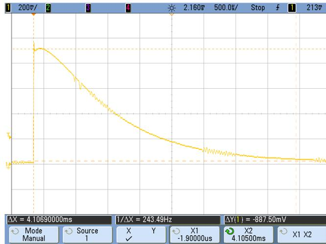
Figure 37. Inrush measurement.
