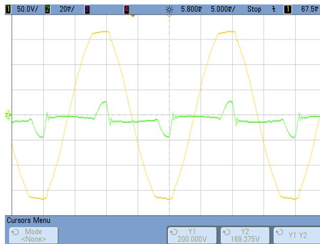
Figure 36. Input voltage and current waveform - 230 VAC.
