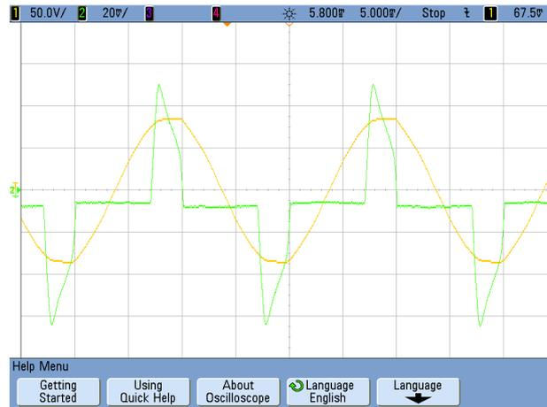
Figure 35. Input voltage and current waveform - 115 VAC.
