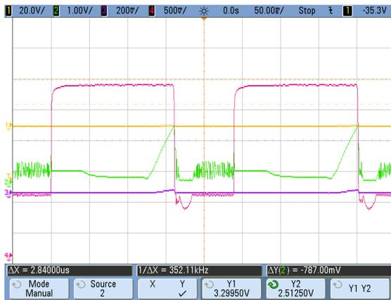
Figure 27. Waveforms while controller loops starting.
