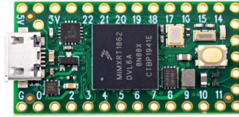
Figure 13. Teensy 4.0 microcontroller unit [43].
