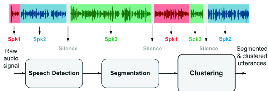
Figure 1. The process of speaker diarization. A typical speaker diarization system consists of a speech detection stage, a segmentation stage, and a clustering stage [3].
